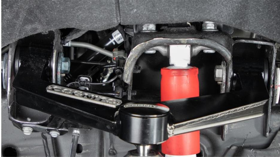
12. Mount the uni-ball pin to the spindle with the supplied hardware. Torque the castle nut to 80 ft-lbs. while ensuring that the cotter pin hole on the uni-ball pin lines up with one of the notches on the castle nut. Insert the cotter pin and bend the ends around the nut to fully secure.
