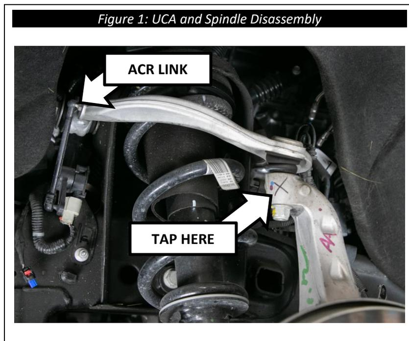
4. Use a 21mm wrench to remove the factory bolts that connect the factory UCA to the frame. Pay attention to the orientation in which they were removed and place the hardware safely aside. These bolts need to be re-installed in the same orientation and location.
