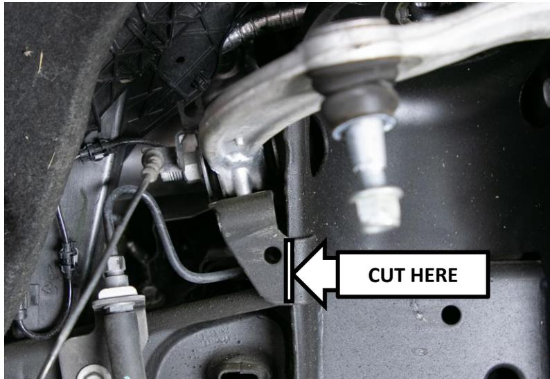
6. Locate the **80012** Cognito Uni-Ball UCA Driver Side Assembly and mount the Cognito UCA to the frame using the factory bolts and nuts. The thrust washers should be on the exposed side of each bushing, see Figure 3.
