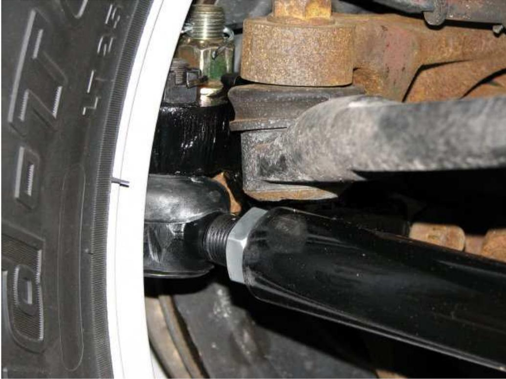
Draglink adjustment. At full turn to the right, the draglink tie rod end, shown in the above picture, may contact the tie rod depending on the rotation of the draglink.
