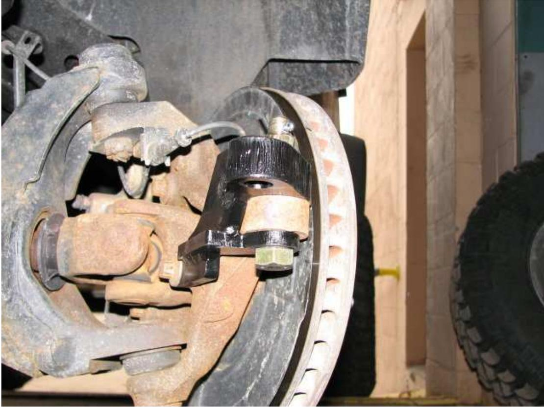
Reinstall the wheel bearing retaining bolt and when that is tightened up the hub should pull into place properly, then tighten the 5/8" bolt. Torque the wheel bearing bolt to 90 ft lbs and torque the 5/8" bolt to 110 ft lbs. Once the 5/8" bolt is tight, the aluminum crush bushing should disappear into the opening as shown in the picture above.
