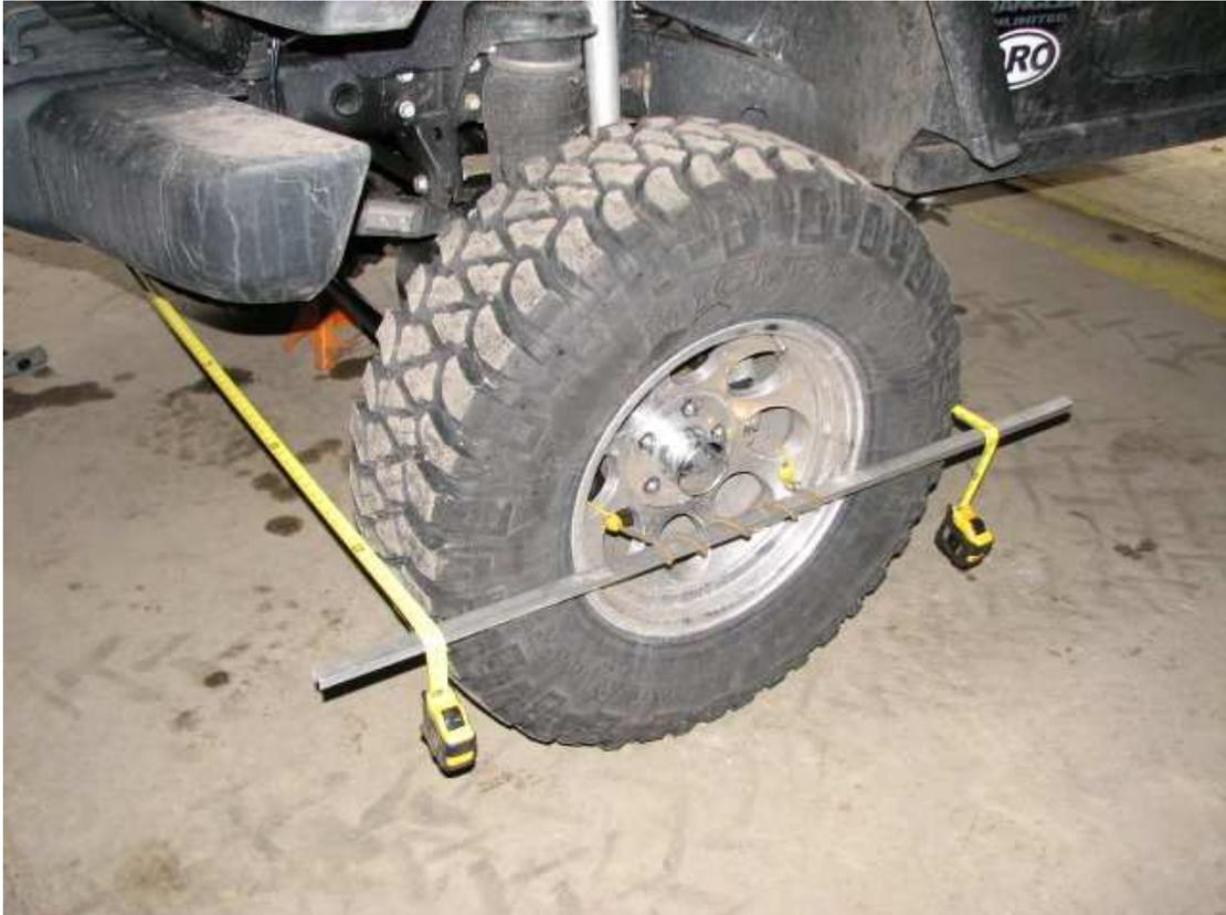
Utilizing a pair of straight edge materials (aluminum C-channel shown, available from most hardware stores) and a pair of bungee cords, attach the straight edges to the wheels as shown. Take care to not bend/deflect the straight edge with the tension of the bungees, but yet you need to have enough tension to keep the straight edges in place.
