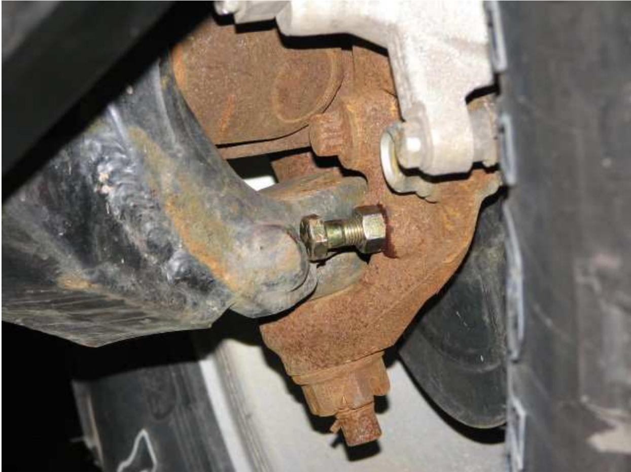
Steering stop adjustment. There are a pair of 3/8" x 1.25" bolts supplied in the kit, with nuts, these are to be used to replace the stock steering stop bolts. Due to the new geometry of the tie rod ends, the outside tire (left tire on a right turn) will turn farther than previous, so we need to adjust the stops to keep the tire from contacting the suspension components.
