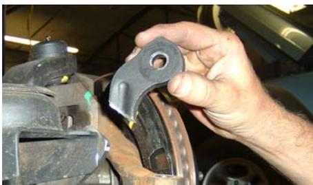
3. Place the new sway bar mount on the inner knuckle so that it is vertical (see last photo), and tack weld it in place. Double check to make sure that the mount is in the right location and then final weld.
