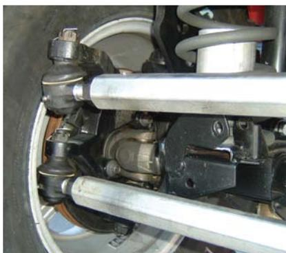
12. Check all bolts and nuts for proper torque specifications, and use cotter pins where required.
