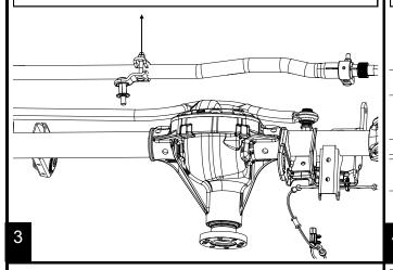
Hint: Slide the stabilizer mount over to the track bar bracket and rotate it until the stud contacts the bottom of the track bar bracket. This will provide a good location to pry on the stabilizer bracket. After prying, slide the bracket to the passenger side of the tie rod. The smaller diameter of the tie rod end will aid in removing the stabilizer mount.
