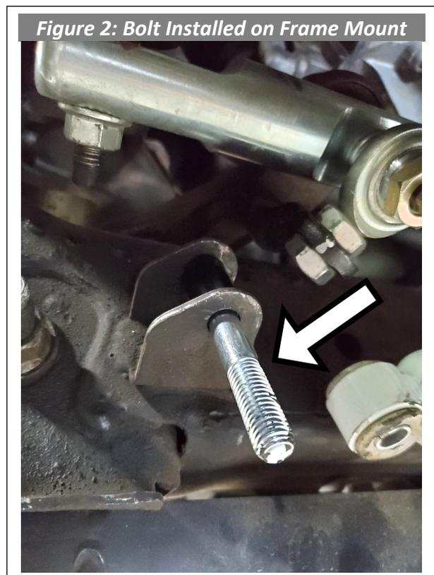
3. From the top, install the supplied 12mm bolt, with one of the supplied washers, through the frame mount and crush sleeve. See Figure 2.
