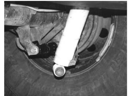
6. Connect the shock to the bracket extension using the new bolt included with the kit.
