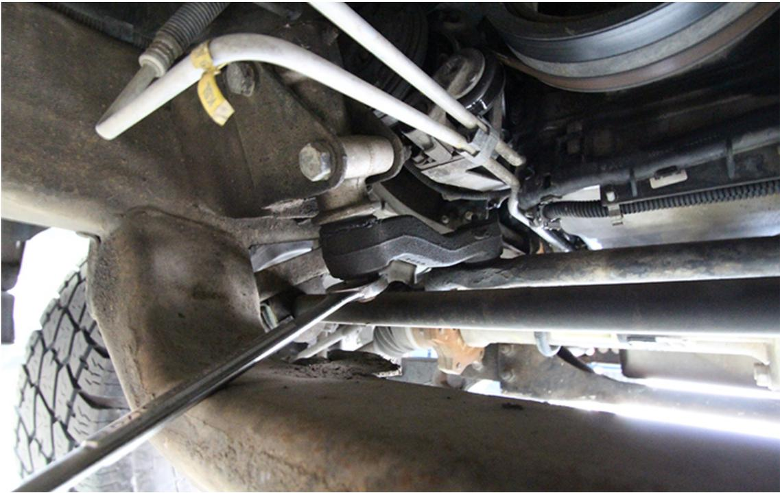
Figure 3: Idler arm bracket installed
