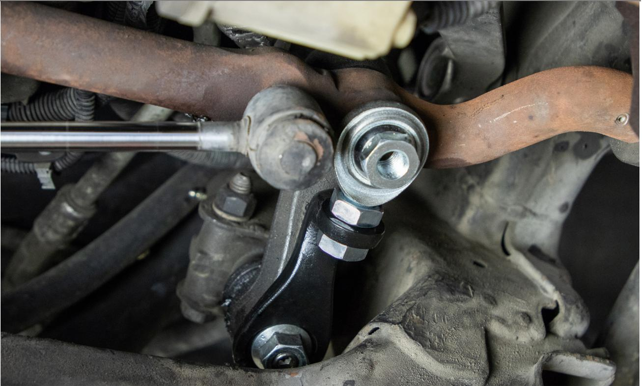
7. Tighten the idler pivot nut to 85 Ft.-lbs. before reinstalling the idler pivot into its frame mounting pocket. Reinstall the two bolts and tighten to 78 Ft.-lbs.
