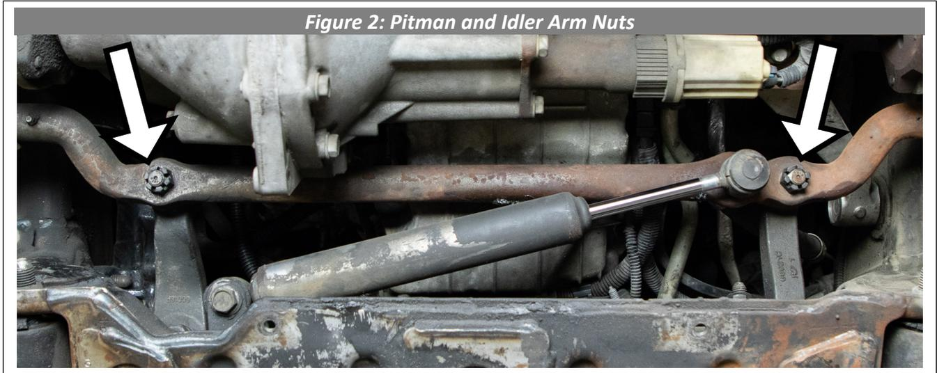
3. Unscrew the large nut holding the pitman (driver's side) arm to the steering box using a 32mm or 1 5/16" boxed end wrench. Remove it and the large lock washer. See figure 3.
