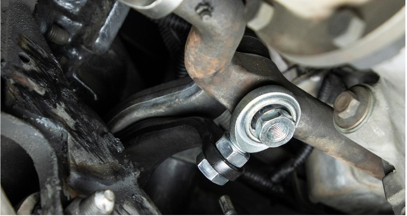
*Figure 7: Idler Arm Bracket Installed*
