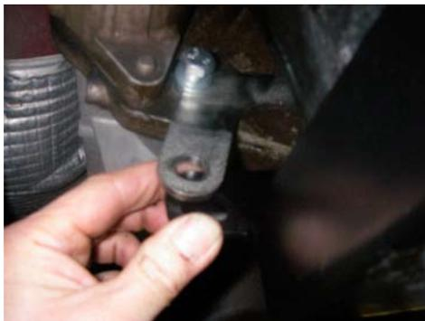
4. On 2003 and newer Jeeps the addition bell housing bracket is used. Hold the bell housing bracket up to the bell housing to see which bolts need to be removed. Remove the 2 factory M10 bolts, install the bracket to the bell housing just finger tight using the supplied M10-1.50 x 25 bolts with flat washers. Put one flat washer between the new bracket and the bell housing to space the bracket away from the thin inspection cover.
