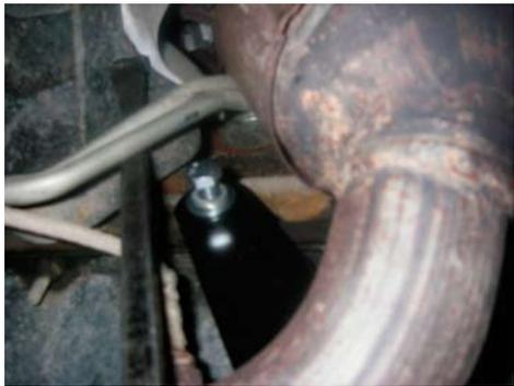
sides but some engine blocks from 1991-1999 will have a metric thread M12-1.25 on the driver side of the block. If your engine has a knock sensor in the 12 mm bolt hole, remove the sensor and reinstall it through the arm on the HD skid plate. Be careful to select the correct bolt for your Jeep. If the bolt bottoms out before it is tight on the skid arm bracket, put an additional flat washer under the head of the bolt.
