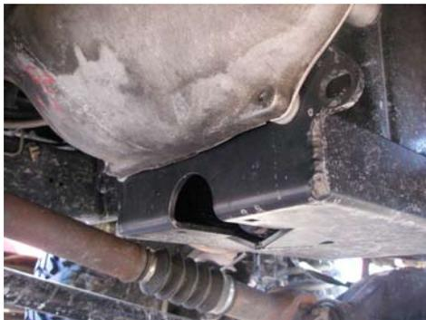
2. Install both engine side bolts first leaving them loose until the bell housing bolts are installed, then move the back of the skid up near the bell housing. Using the bolt holes on the skid, remove the corresponding factory bolts and move the skid up into place.
