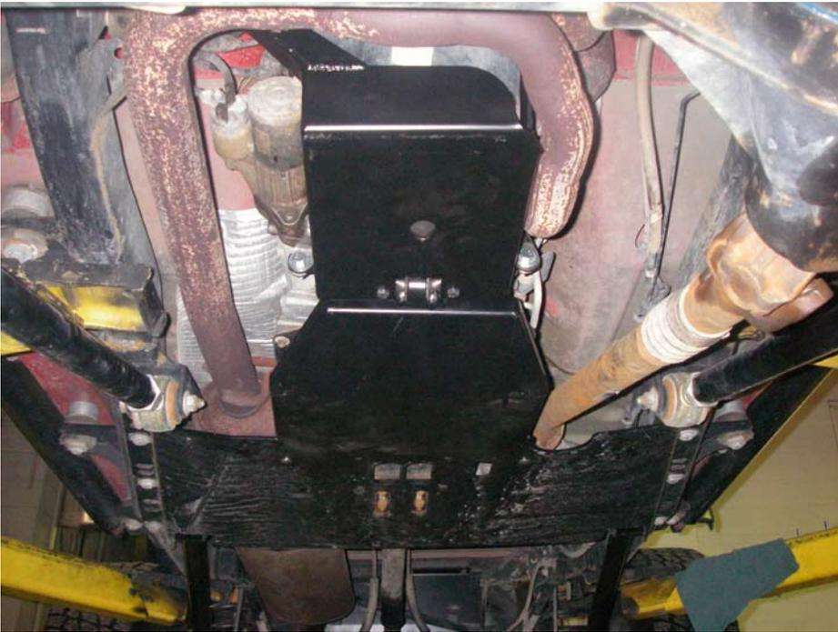
On a TJ Wrangler the engine oil skid along with the HD transmission skid and Belly Up skid plate provide protection to all vital components when operating in rocky terrain.
