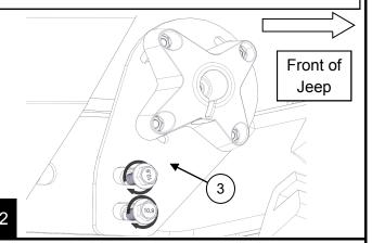
Install the Mud Flap Assembly(1) into the indexed Mud Flap Mount and turn the knob clockwise 3 to 4 times to make sure it will not fall out while adjusting the mount.
