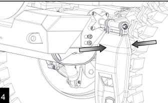
The Transit Mud Flaps are easily removable by simply unthreading it from the Mud Flap Mount using the Mud Flap's end Knob
