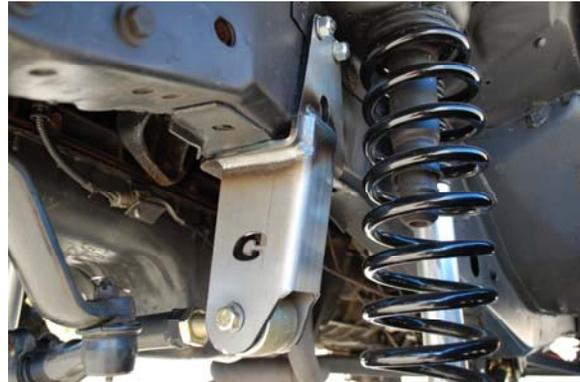
27. Bolt into OEM location reusing the OEM bolts and tighten all bolts to factory specs.
