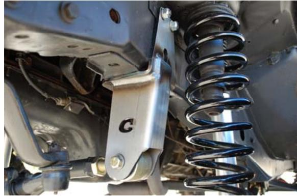
5. Bolt into OEM location reusing the OEM bolts and tighten all bolts to factory specs.
