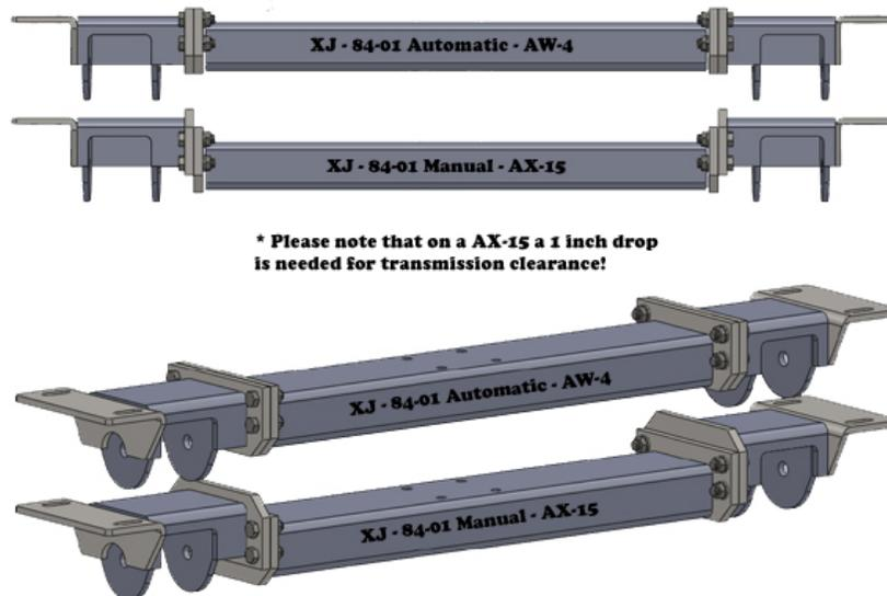
8. Center the new cross member and secure it using the two mounting holes on each side.
