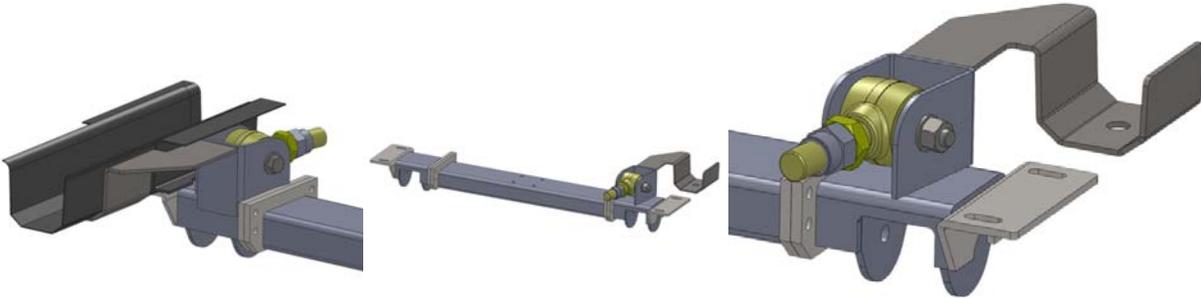
12. Route any fuel or brakelines below the 3 link brace. Shown below left is the 3 link brace ready for welding.
