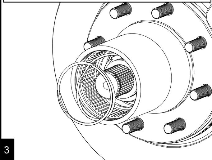
Slide the outer spline into the hub by compress the spring. Note the orientation of the outer spline with the engagement teeth facing out.
