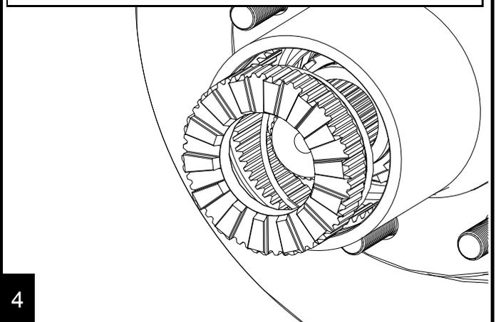
Apply grease to the bronze bushing, slide the inner spline over the axle shaft. Rotate the hub to ensure the inner spline and outer spline interlock. Note the orientation.
