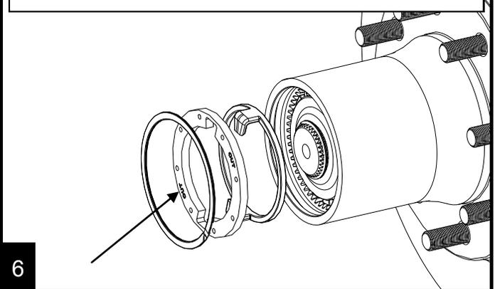
Push the dial out of the bezel and apply a coating of grease to the O-ring and O-ring groove in the bezel. Carefully reinstall the dial into the bezel to prevent the O-ring from being damage.
