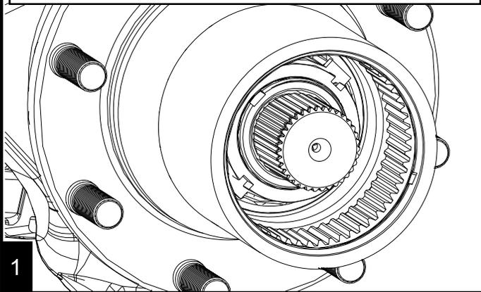
Install the spacer over the stub shaft.
