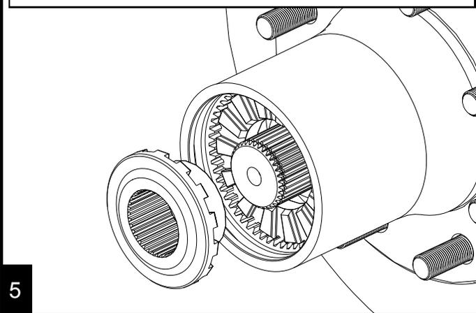
Install the disengagement ring and bolt ring. Install the full circle, internal retaining ring into the hub. **Note: Place the "OUT" on the bolt ring faces out. Be sure the retaining ring seats completely.**
