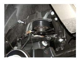
7. Reinsert the yellow urethane bumpstop and reinstall the rear coil spring.
