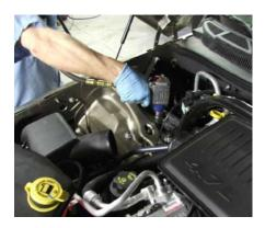
3. Remove the fasteners and move the Power Distribution Center to gain access to the driver side strut upper mounting nuts. *Do not disconnect the wires*.
