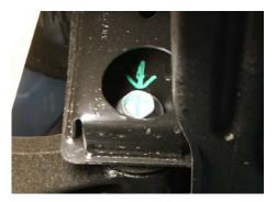
Attach the lower end of the strut and use the floor jack to raise the control arm and strut up into place, then install the 4 upper nuts. Reinstall the control arm lining them up the cam bolts as near as possible to the original location.
