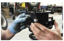
13. In order to install the strut with the 2 inch spacer it is necessary to remove the lower control arm mounting bolts at the sub frame. Mark the position of the bolts and remove them to allow the lower control arm to drop down just enough to install the longer strut. Do not completely remove the control arm or knuckle.
