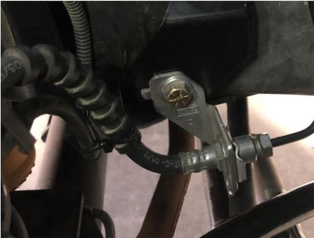
*Figure 6: Passenger Side ABS Line Routing*
