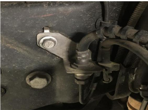
*Figure 1B: OE Brake Line Bracket, Bolt Removed*
