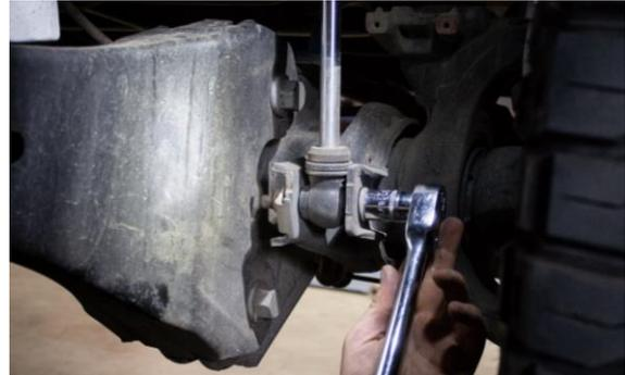
9. Properly position and check to ensure that all brake lines, vacuum lines, hoses, and wiring are free to lift vehicle. Raise the vehicle slowly until the front spring preload is removed (Figure 9A). DO NOT raise the vehicle any higher than necessary to remove springs. This could result in driveline, wiring, brake line, and suspension component damage. Remove front springs and rubber isolator from the driver and passenger side spring perch (Figure 9B).
