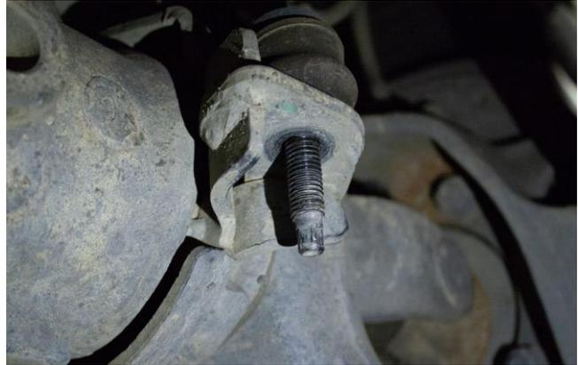
8. Remove the front shocks from both driver and passenger side of the vehicle (Figure 8 A/B)
