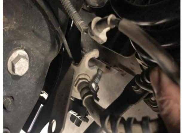
3. Install the Cognito brake line brackets (Part # 8546 & 8545) to the frame by inserting the alignment tab into alignment hole and rotating the bracket mounting hole into position. Attach to the frame using the OE bolt removed in step 1, and torque to OE torque specifications (Figures 3 & 4).
