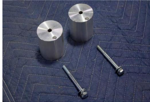
12. Insert the locking tab on the OE bump stop mount into the alignment hole on the bump stop spacer (Figure 12- image shows a different size spacer). Using (1) M8x1.25x80mm Lg. cap screw, assemble with (1) 5/16" lock washer between the bolt head and (1) 5/16" SAE flat washer. Orientate the spacer so that the flat side of the bump stop mount is facing the spring (Figure 13 – image shows a different size spacer) and torque to 25 ft.-lbs.
