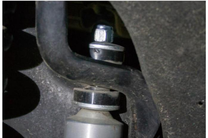
16. Before starting this step, it is recommended to get another person to assist you. Align both front shock bottom eyelets into lower shock mount shackle. Slowly lower the vehicle until the lower shock eyelets are aligned with the shackle mounting hole (Figure 16A). Re-install the OE bolt and locking nut plate, then torque to OE torque specifications (Figure 16B).
