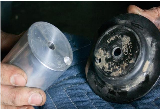
Figure 13: Bump Stop Spacer Orientation
