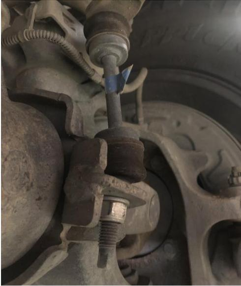
*Figure 7B: OE Sway-Bar End Link, Nut Removed*
