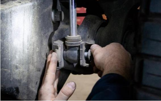
*Figure 16B: Front Lower Shock Mount Installed*
