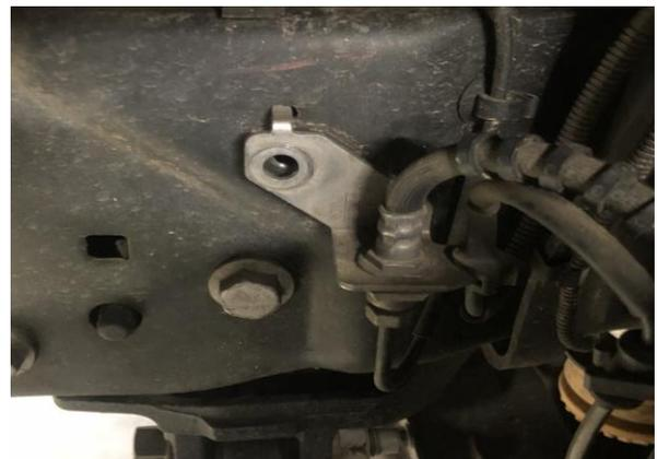
2. Remove the ABS line from both driver and passenger side OE brake line brackets by pulling the rubber boot out of the containment slot (Figure 2 A/B).
