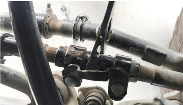
*Figure 17B: Steering Link Adjuster Secure*
