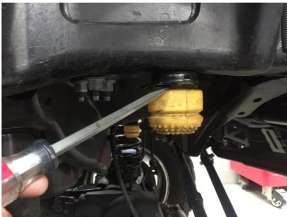
*Figure 10B: FSD Bump Stop Spacer Hardware*
