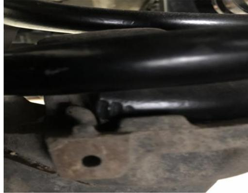
15. Once the springs are installed, locate the Cognito/FOX extended length shocks. Remove the top washer (Figure 15A) and bushing, then insert the top shock mounting stud through the frame, making sure the polyurethane pancake bushings are in place on both sides of frame. Install the top mounting washer with the concave side against bushing (Figure 15B). Repeat for the opposing side front shock, but do not tighten at this time.
