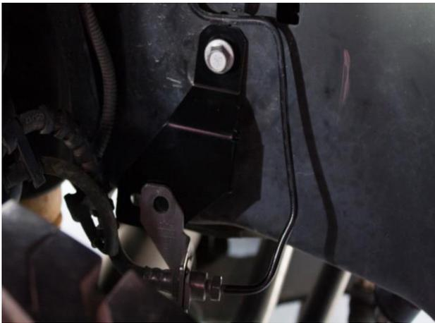
*Figure 4: Driver Brake Line Bracket*
