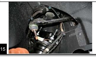
Attach the bottom of the fork to the lower A-arm with the factory bolt. Torque the bolts to factory specifications. **TIP:** A hydraulic jack is a convenient way to raise the knuckle into position so that the upper A-arm can be connected to the knuckle. Torque to factory specifications.
