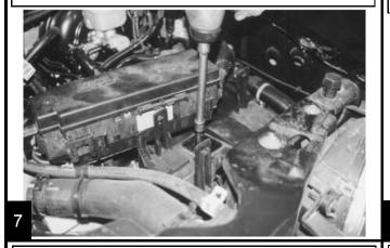
The connectors that attach the wires to the tray can be easily disconnected. Disconnect the battery sensor from the bottom of the battery tray.
