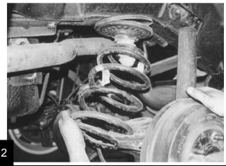
Position the polyurethane spring spacer on the axle's lower spring pad after removing the bottom factory rubber insulator.
