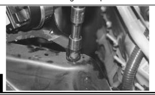
Disconnect the upper end of the strut assembly by removing the four nuts that secure it to the body compartment.
