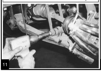
Use a 21 mm socket to remove the bolt that secures the top of the fork to the bottom of the strut assembly.
