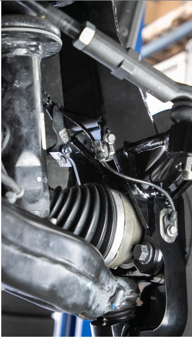
Figure 51a: Wheel Speed Sensor Installed (2019 model shown)
