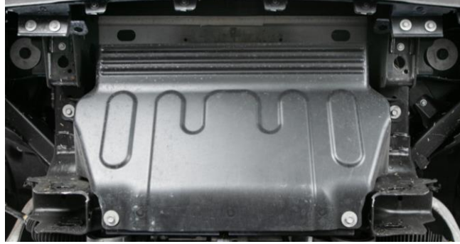
Figure 33: OEM Front Skidplate Reinstalled
