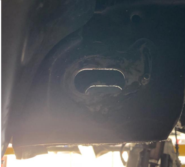
Figure 24g: Driver's Side Front Crossmember, After Trimming
