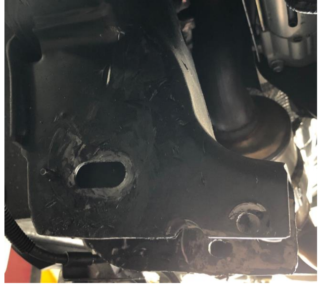
Figure 24f: Passenger's Side Rear Crossmember, After Trimming
