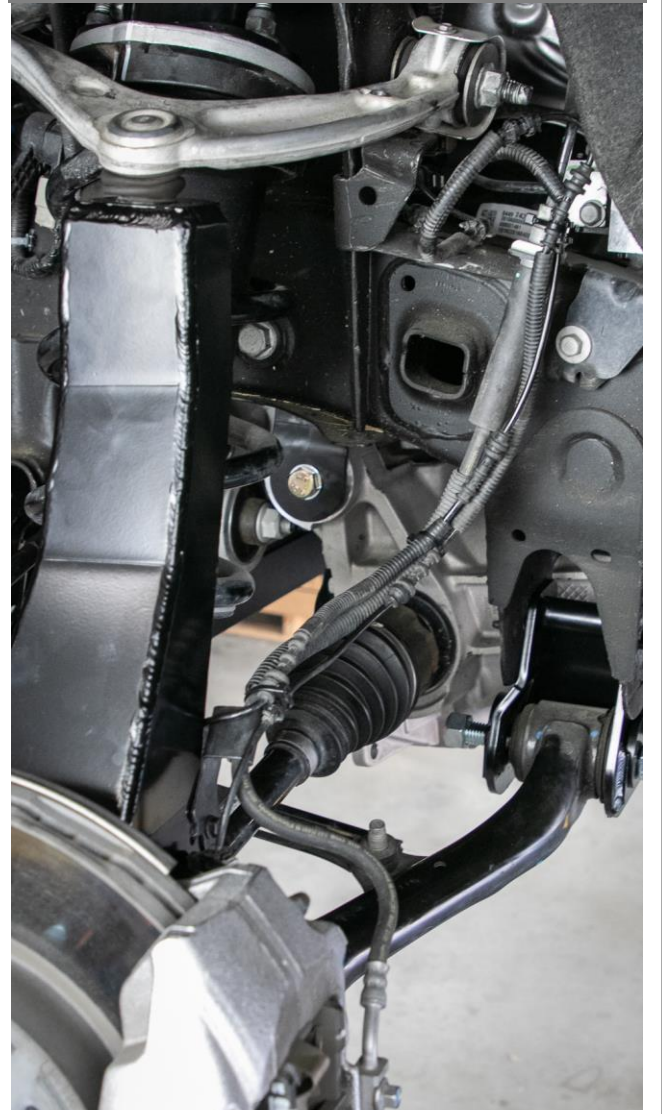
Figure 51b: Wires Cable-Tied Together (2019 model shown)
