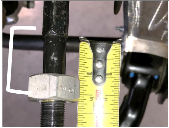
Figure 46b: Measure Position of Die
