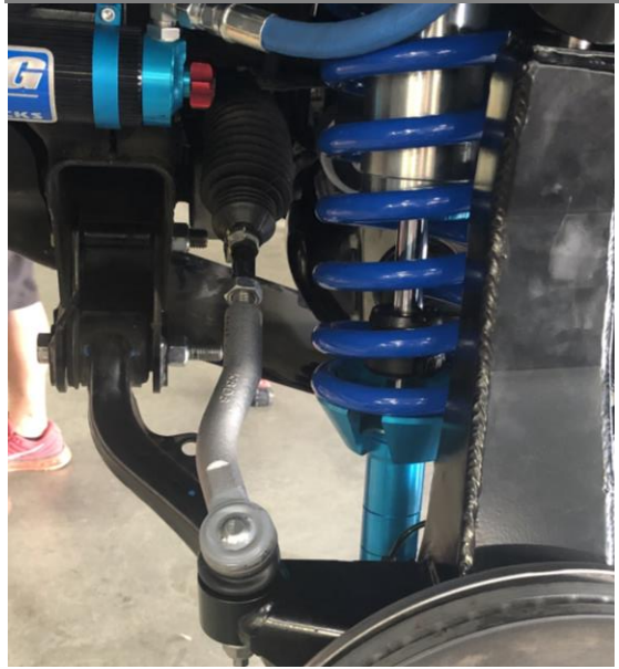
Figure 46d: Tie Rod End Installed (Driver's Side Shown)
