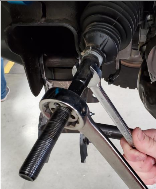
Figure 46a: Thread Die On To Tie Rod End
