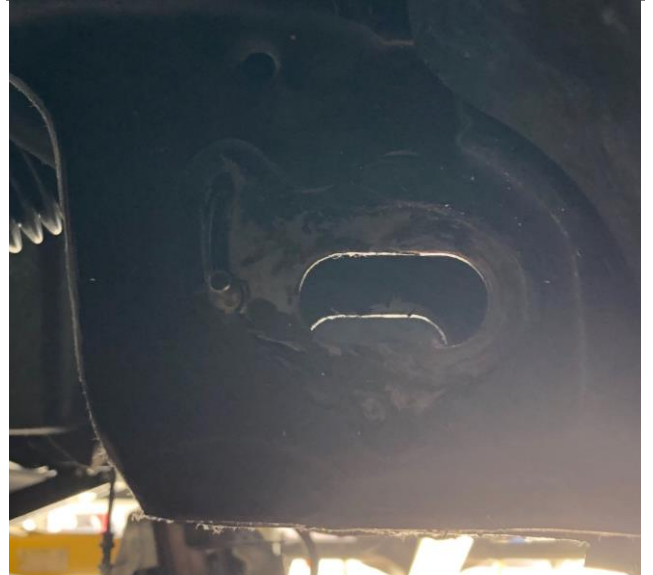
Figure 24h: Passenger's Side Rear Crossmember, After Trimming
