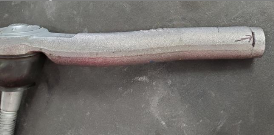
Figure 46c: Cut Outer Tie Rod End
