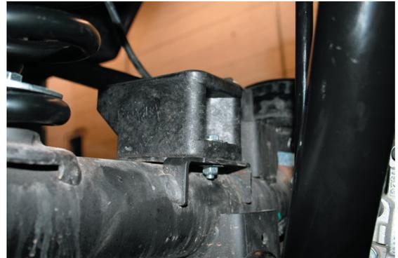
19. To install the rear coil spring retainers on the bottom end of the coil springs first insert the flanged nut into the provided wrench tool, as shown below, and put the nut under the spring pad.
