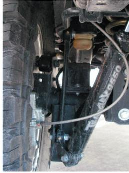
21. Install the rear trackbar bracket at the frame.
