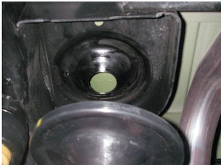
13. If you plan to carry a lot of weight in the rear of the vehicle, reinstall the factory spring isolator onto the TeraFlex spring spacer/guide, otherwise leave it off. **Note:** The factory spring isolator can be added in later if you add a full size spare tire or if for any other reason you want to slightly raise the back of the vehicle.
