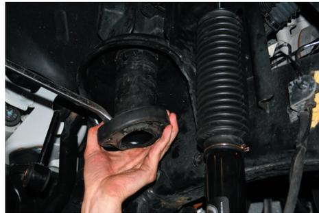
35. Install the new front spring spacer.
