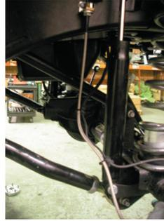
33. Remove the factory upper bump stop from the cup on the bottom of the coil tower.
