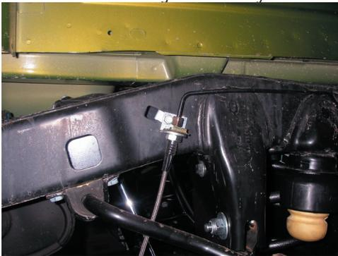
24. Anchor the new rear brake hoses with the angle brackets and clips provided in the hardware kit.
