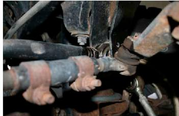
25. Install the new track bar that comes with the 5 inch Pro system and move on to final assembly.
