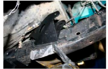
22. Weld the bracket to the frame and paint the weld area to prevent rust.
