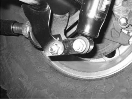
Install the extended brake line hose Figure 8 and the extended sway bar links. Mount the extended brake line tee on top of the truss and reconnect the hard lines. Rear installation is complete.
