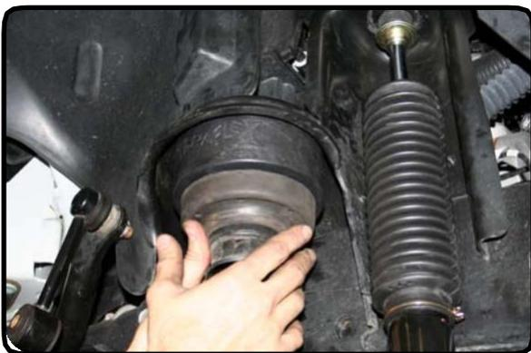
28. Using grease, lube the bump stop extension to install it into the spring tower. (You may need a piece of wood or equivalent to put in between the extension and the coil perch and jack up the axle to install extension. Do one side at a time.
