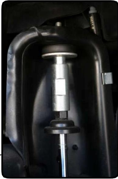
32. Install factory rear sway bar links in the front on the outside of the sway bar and inside of the axle mount. Torque to 75 ft-lbs.
