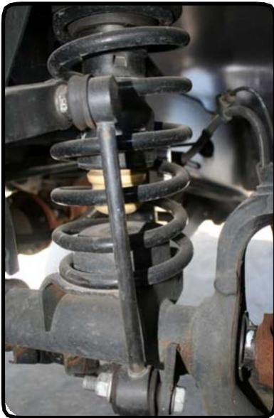
33. Reinstall wheels, torque lug nuts to 95- 115 ft-lbs, Remove jack stands, lower the vehicle onto its own weight, and torque all the control arm bolts. Torque the uppers to 75 ft-lbs and the lowers to 125 ft-lbs.
