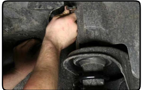
24. Remove sway bar links using 18mm socket and wrench at the axle and 18mm socket and 20mm wrench at the sway bar. Lower the jack enough to remove the springs.
