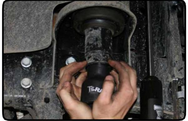
29. Use grease to lube the yellow bump stop and install it into the extension.
