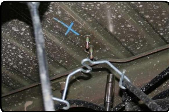
11. Carefully lower the rear axle far enough to remove the rear springs. Be careful not to let the coils fall out as you lower the axle. Lower the axle far enough to install the new 2.5" spacer in place. While lowering the axle make sure the brake lines, ABS wires and axle vent do not stretch as this could cause damage to these vital parts.
