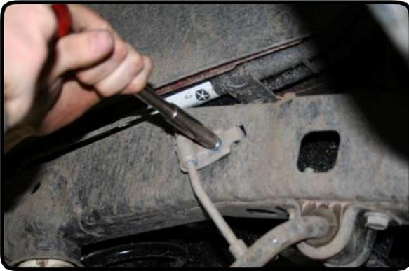
10. Remove and discard the bracket that holds the park brake cables to the body using a 10mm deep well socket.
