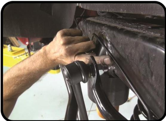
17. Install new rear bump stop spacer by placing the spacer on the axle pad lining up both holes with the overhang part of the pad facing forward. Use the provided 5/16" x 1 1/4" bolts with 5/16" washers and 5/16" nuts. Tighten with 1/2" wrenches.
