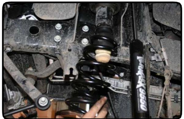
31. If your kit comes with the shock adapters install the front upper shock adapter by spinning it onto the factory shock using red thread locker . Then install the provided washer then the original rubber bushing with the big hole in it and use the other one on the upper side of the frame and install in the same order it was removed. Torque to 20 ft-lbs on the frame side and 56 ft-lbs on the axle side.
