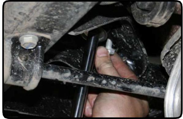
7. Remove sway bar links using an 18mm socket and wrench, make sure to put aside for use in the front of the vehicle.
