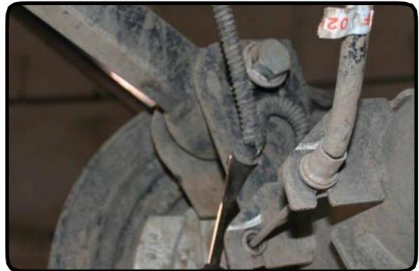
9. Disconnect the brake line bracket at the frame using a 10mm socket. **DO NOT DISCONNECT THE BRAKE LINES FROM THE CALIPERS.**
