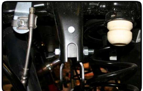
14. Install the factory isolator onto the new TeraFlex rear spacer. Install the new spacer into the frame. You should feel or hear a popping and the spacer should stay hanging from the frame.
