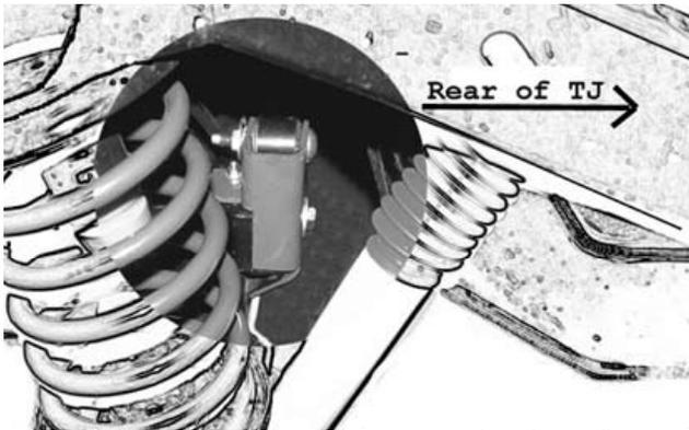
16. With the track bar bracket in place, the two (2) smaller holes in the bracket should line up close to the holes in the axle bracket vacated by the plastic shield removed in Step 13.
