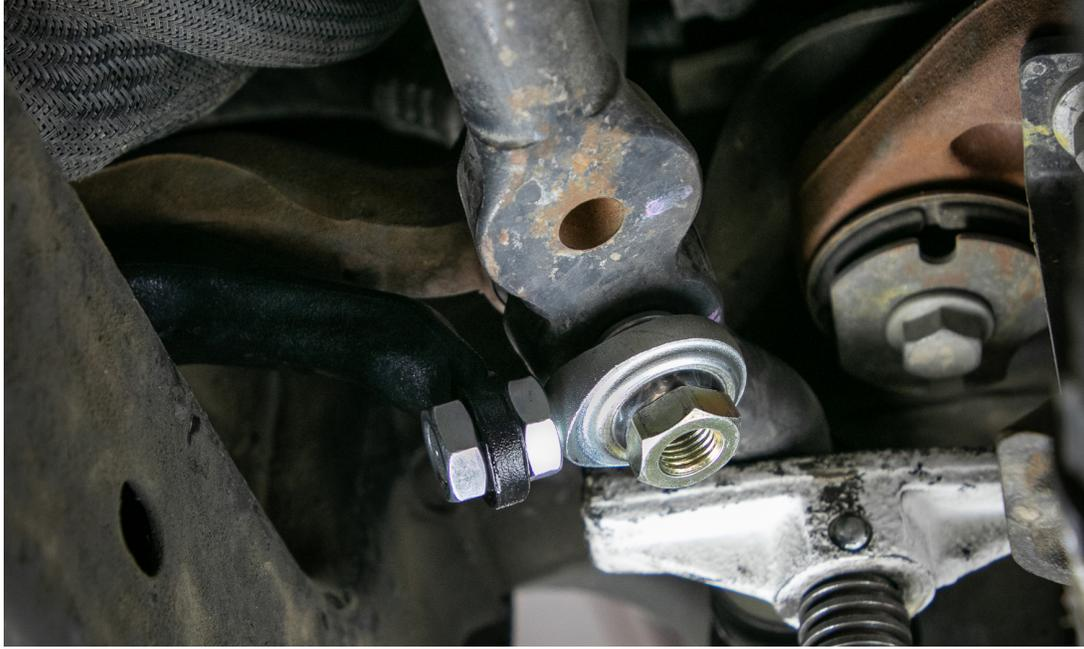
10. Reinstall the idler pivot into its frame mounting pocket and reinstall the two bolts, tightening to 122 Ft.-lbs. Then tighten the idler pivot nut to 200 Ft.-lbs.
