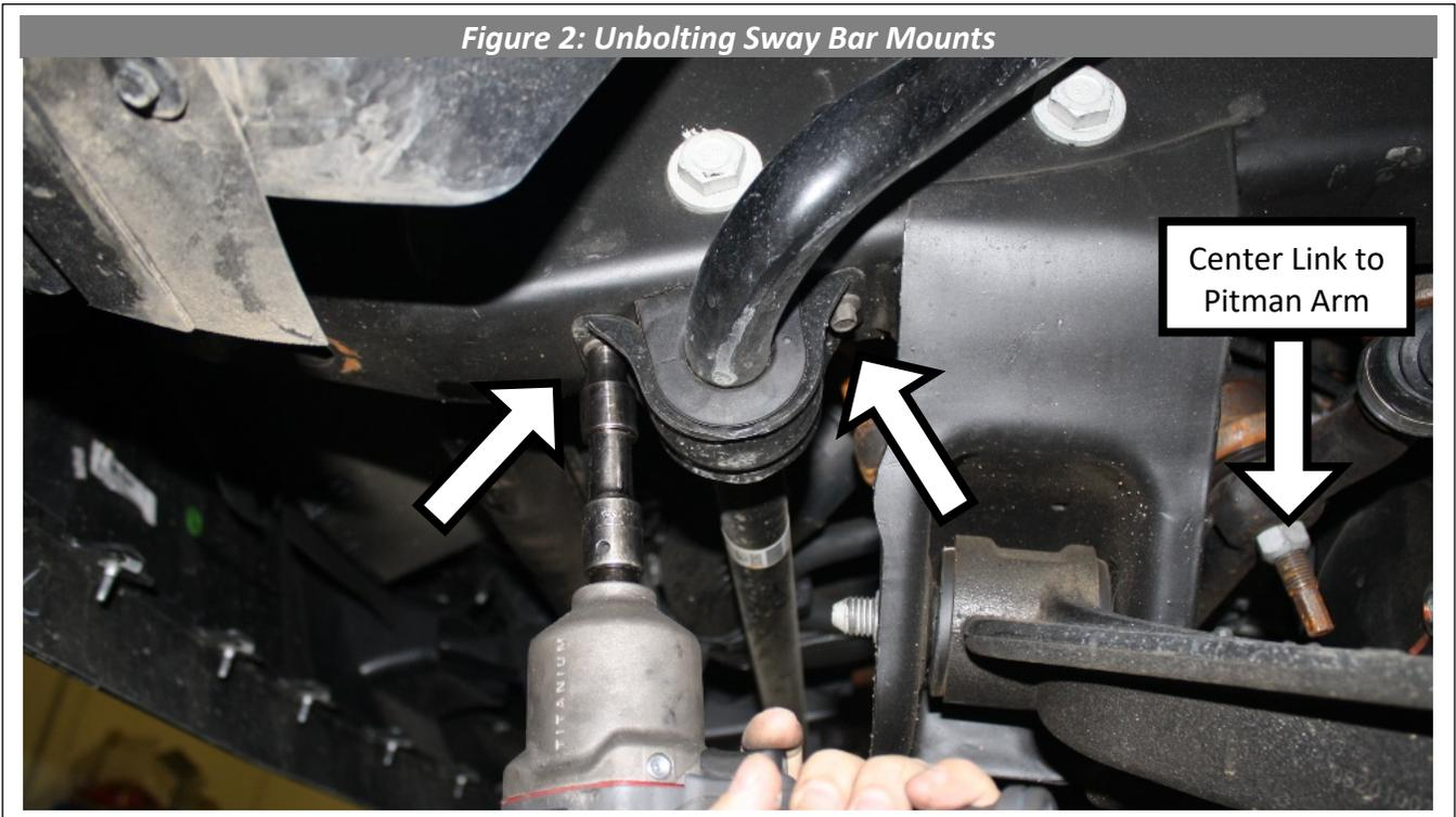
3. Unscrew the factory lock nuts that hold the center link to the pitman and idler arms, using a 21mm deep socket, and discard them. See figure 2.
