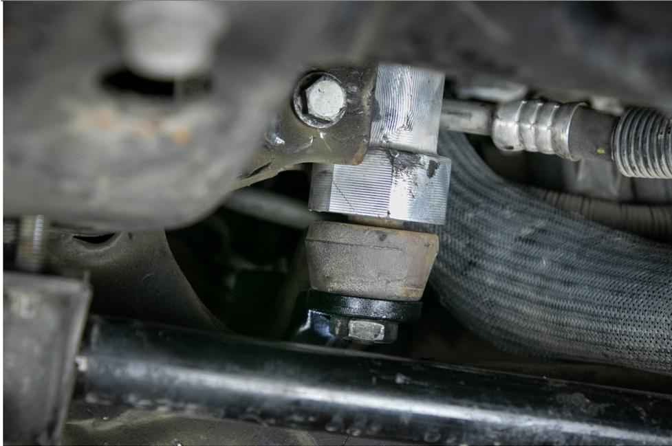
11. Reinstall the three bolts which hold the steering box to the frame, tightening the bolts to 203 Ft.-lbs.
