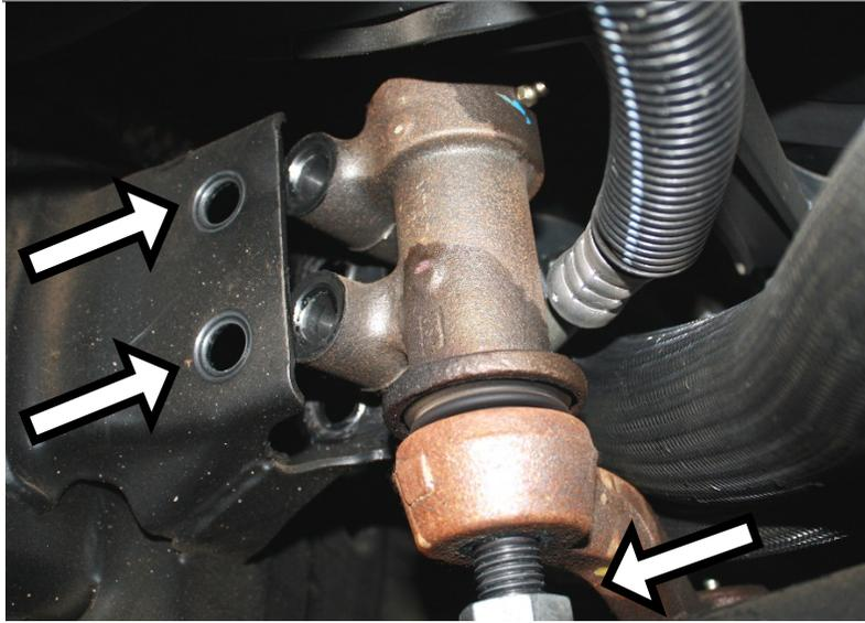
**Note:** There are two different center link designs used by GM, one with the rubber isolator bushing shown below, and one without. If your center link has a rubber bushing as shown, discard 6402 spacer included in the kit.
