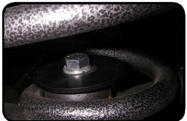
16. Install new rear sway bar links on the inside of the sway bar and the inside of the axle bracket. Use the factory bolt on the axle side with the nut on the outside so excess threads will not interfere with the shock. Use the provided 12mm bolt and washer for the top side with the 12mm nut and washer on the inside to give the most possible room for tire clearance. Torque to 75 ft-lbs.
