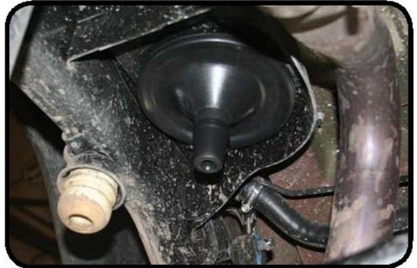
13. Install the factory isolator on the new spring guide spacer. Don't forget to reuse the factory spring isolator. If the isolator is left out your ride height will be about 1/2 inch lower in the rear. The isolator also helps dampen noise.
