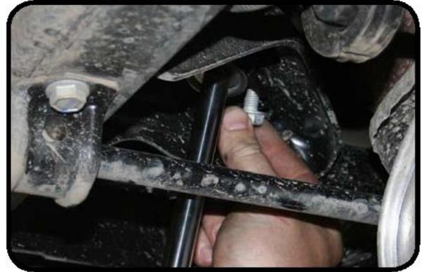
7. Remove sway bar links using an 18mm socket and wrench,
