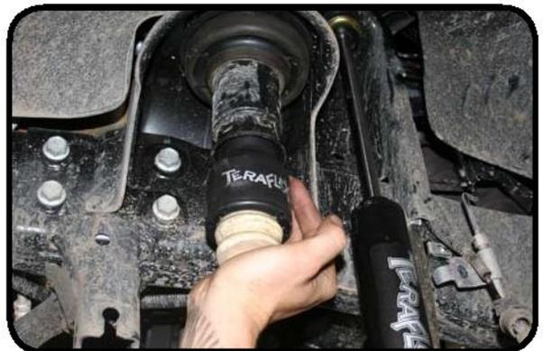
29. Install new 3 inch coil springs. Do the drivers side first.
