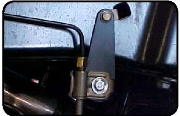
19. Install the new rear track bar bracket by removing the lower control arm bolt. Place the bracket into place, reinstall the control arm bolt. Install the supplied bolt and sleeve into the factory track bar location. Using the supplied u-bolt and nuts install the u-bolt around the axle tube. Torque the u-bolt nuts to 85 ft-lbs and the supplied bolt to 75 ft-lbs.
