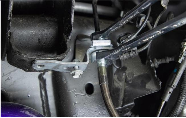
Figure 30: Cognito Extended Stainless-Steel Brake Lines
