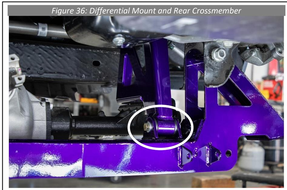
48. Locate the **HP9045** bump stop hardware pack, and install the bump stops to the bottom pads of the Cognito rear crossmember. Torque the bump stop hardware to 18 ft-lbs.
