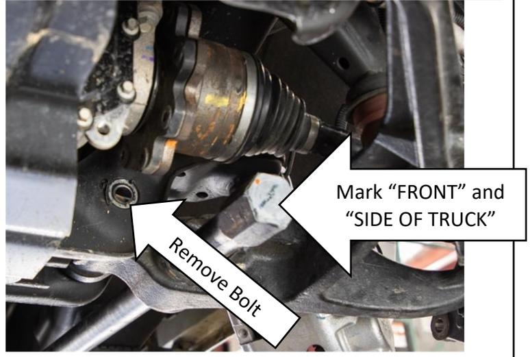
14. You can now remove the torsion bar but **make sure to mark them in their correct orientation and vehicle side they were removed from.**
