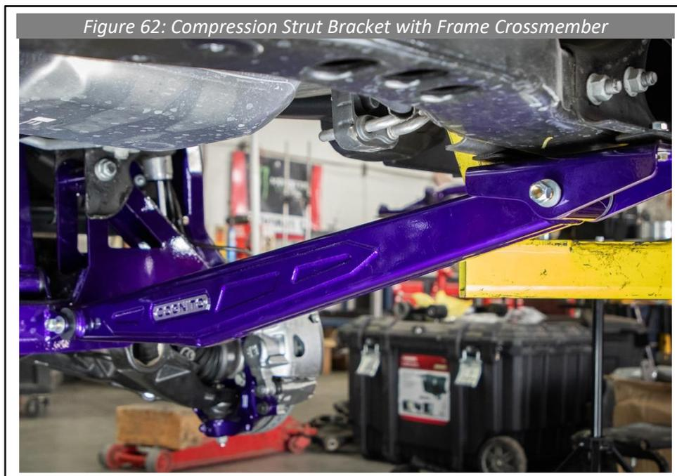
87. After bolting the bracket to the frame crossmember, remove the compression strut from the bracket, and drill the second mounting hole.
