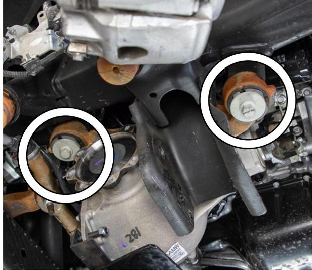
Figure 24: Lower Differential from Vehicle
