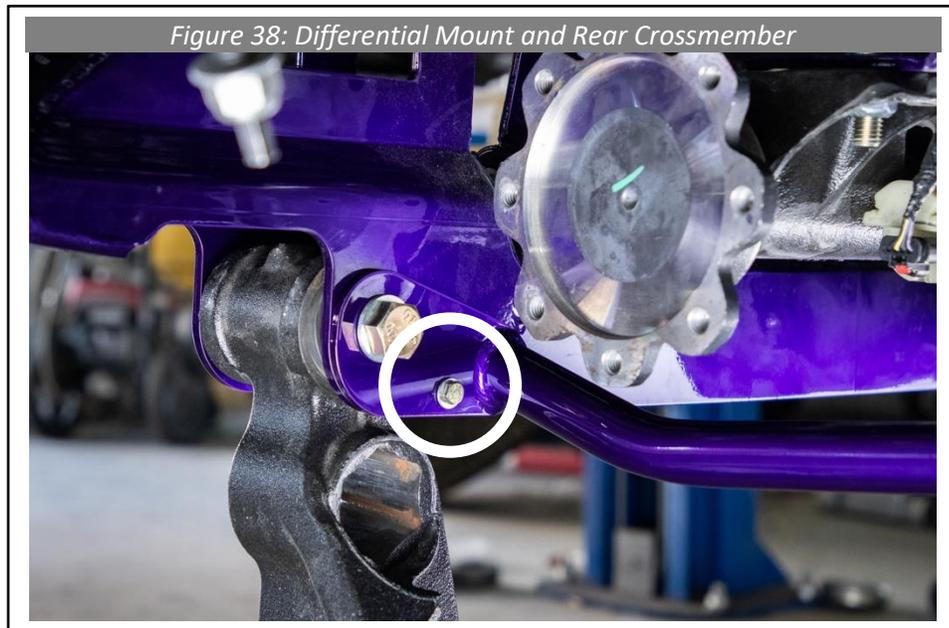
51. Locate the **8765** passenger sub-frame connector and mount the passenger sub-frame connector to the rear cross member following the directions listed in the step above.
