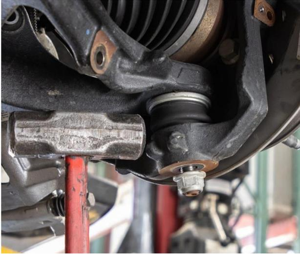
Figure 11: Remove Rear LCA Bolt, Axle, and Torsion Bar
