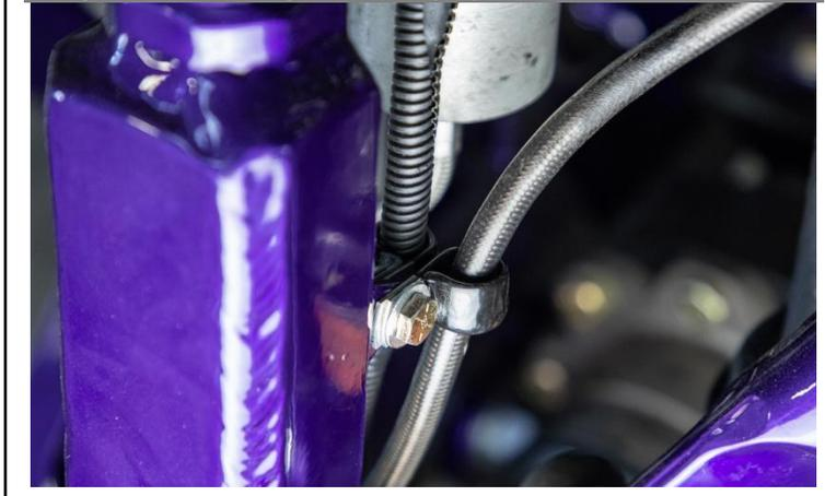
77. For the passenger side, attach the second p-clamp around the brake line and the second p-clamp around the wheel speed sensor to the middle spindle tab in a similar manner as the previous step (see Figure 55).
