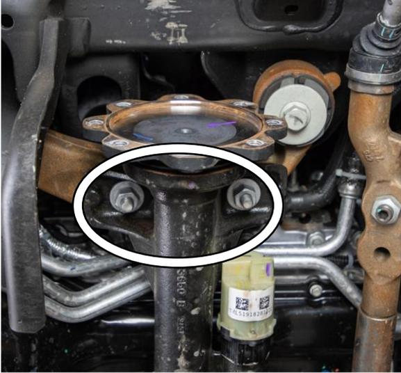
Figure 23: Driver Side Differential Mounting
