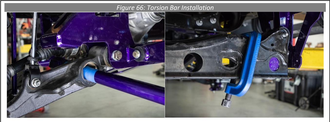
96. Adjust the torsion bars using the adjuster nut and bolt so that the front ride height is even on the passenger and driver side (see Figure 67). Do not over crank the torsion bars to try and gain too much height. **Never tighten the torsion key adjuster screws while the vehicle is on the ground.**
