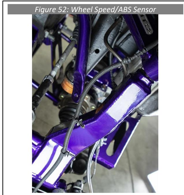
73. Remove the black plastic sleeve from the harness to expose the silicone wire sleeve. Cut the wires approximately 6" from the rubber mount (see Figure 53).
