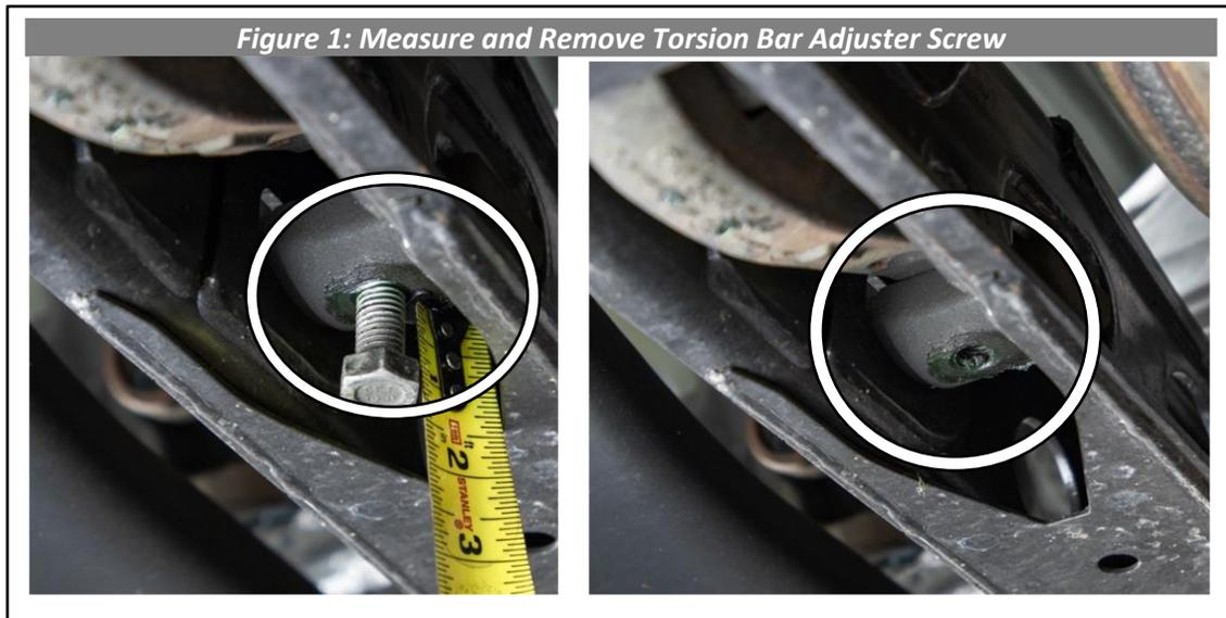
3. Using a torsion bar loading tool, load torsion bar (See Figure 2) and remove adjuster nut (See Figure 3), then unload torsion bar and remove tool. Do this on both sides of the vehicle.
