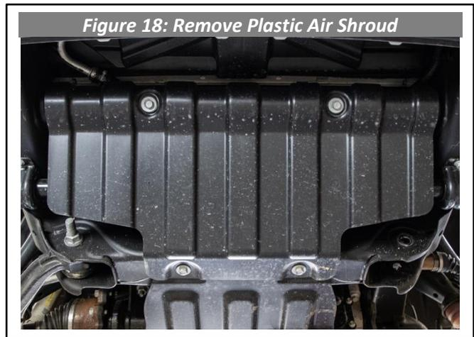
21. Remove the black plastic air shroud from underneath the radiator with a 15mm wrench. This will be re-installed so keep the shroud and hardware (See Figure 18).
