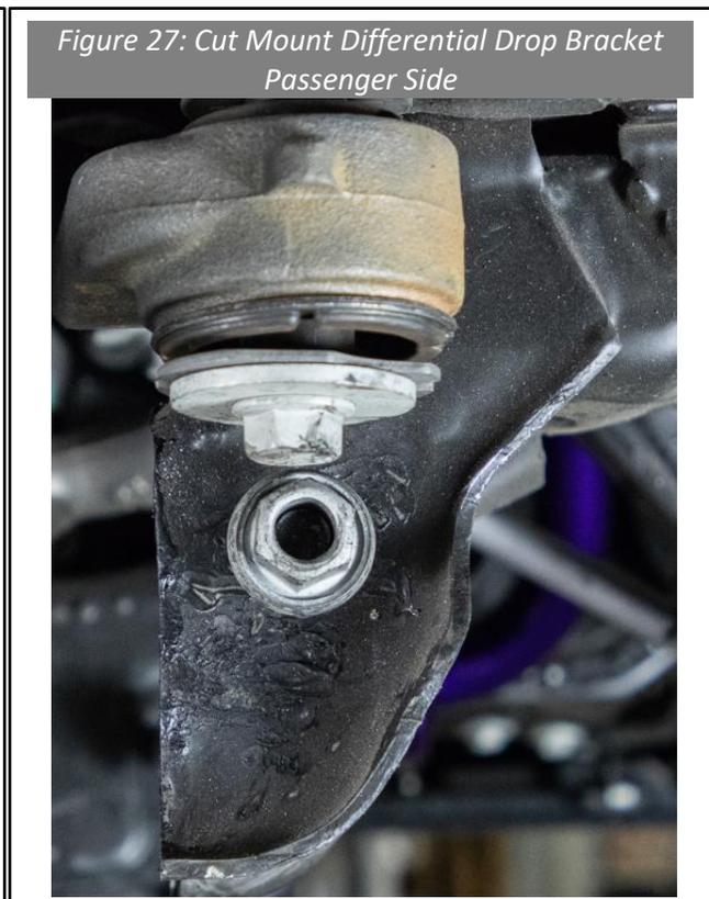
29. This step will begin the installation process. **Do not tighten any fasteners until instructed.** Unless otherwise specified, flat washers will always be used under the heads of bolts and under nuts. Therefore, one bolt with one nut will require 2 flat washers.
