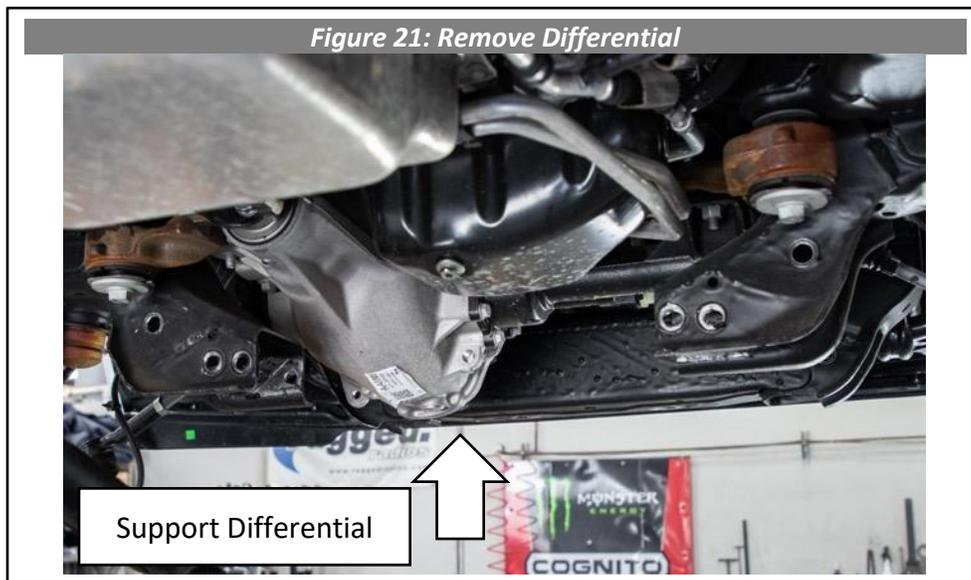
26. **Skip this step for 2WD vehicle.** Loosen, but do not remove the two nuts from the studs on the passenger differential mount with a 21mm wrench (See Figure 22). Then unbolt the driver side differential mount from the frame with a 21mm wrench, leaving the differential mount on the differential (See Figure 23). Then remove the 2 nuts from the passenger side and lower the differential out of the frame (See Figure 24)
