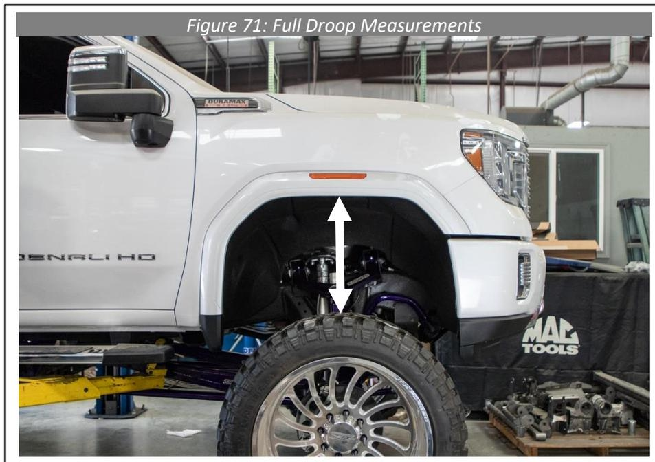
104. Set the vehicle on the ground and drive the vehicle backward at least 10 feet, and then forward at least 10 feet to allow the suspension to settle into place at ride height. Measure from top of tire to fender well and write the measurement here:
