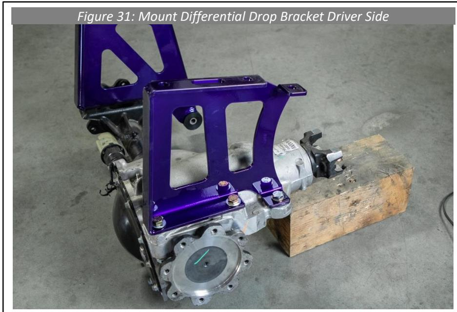
41. **Skip this step for 2WD vehicle.** Bolt **8297** Cognito passenger differential mount onto the front differential in the orientation with the 9/16" hardware from hardware package **HP9121** and a 13/16" and 7/8" wrench. The differential has slotted holes, center the Cognito bracket onto the slotted holes and torque fasteners to 60 ft-lb (See Figure 32). On some trucks it might be necessary to slightly grind on the OEM slotted hole.
