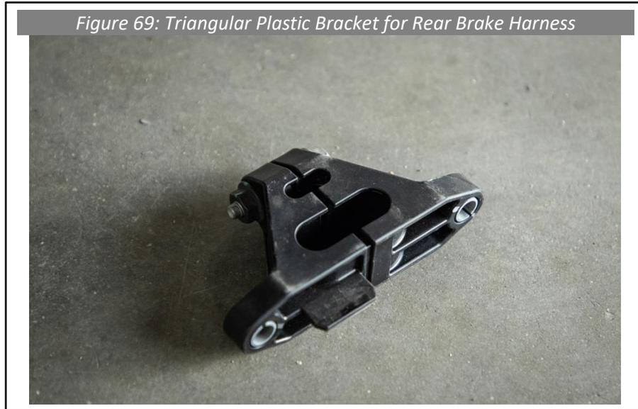
100. Remove these two triangular brackets from the bracket mounted to the top of the rear differential, and from the bracket under the body of the truck (see Figure 70). This will prevent tension on the emergency brake harness.
