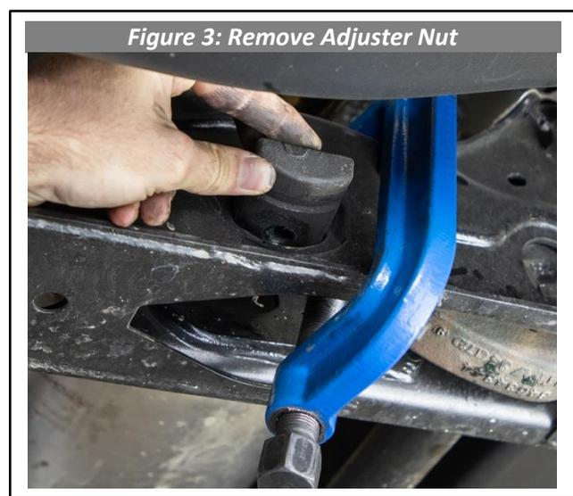
4. Suspension torsion bars hold a lot of energy and both sides of the front suspension are connected through the sway bar. If one torsion bar is loaded, it will affect both sides of the suspension. Unloading them both first is safe practice.
