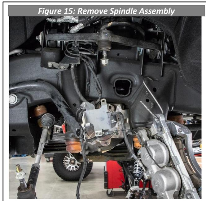
19. Remove the upper control arms at this time using a 24mm wrench but **keep track of the hardware and the orientation it was removed for reinstallation.** Leave the plastic alignment inserts in the hardware (See Figure 16).
