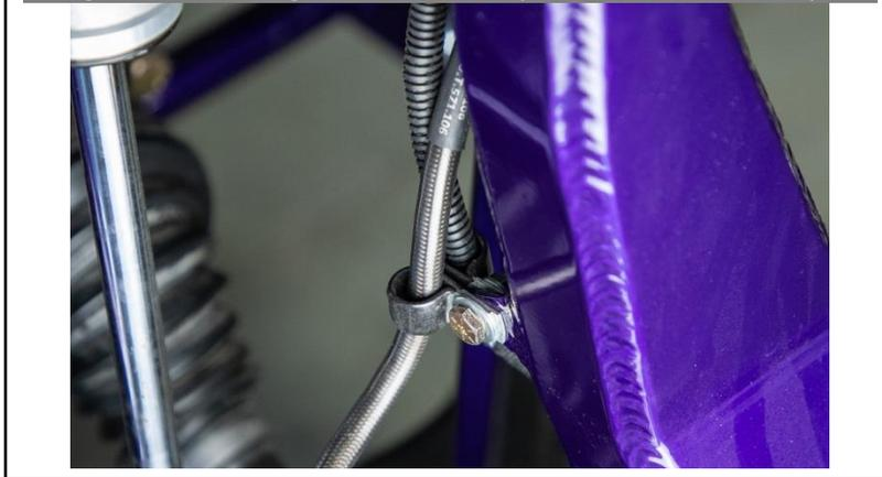
78. For the passenger side, attach the final p-clamp on the wheel speed sensor to the bottommost spindle tab.
