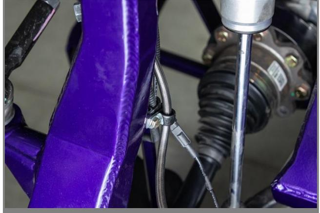
80. After the p-clamps are fastened and tightened down, insert the wheel speed sensor into the side of the spindle and tighten the bolt to factory specifications.
