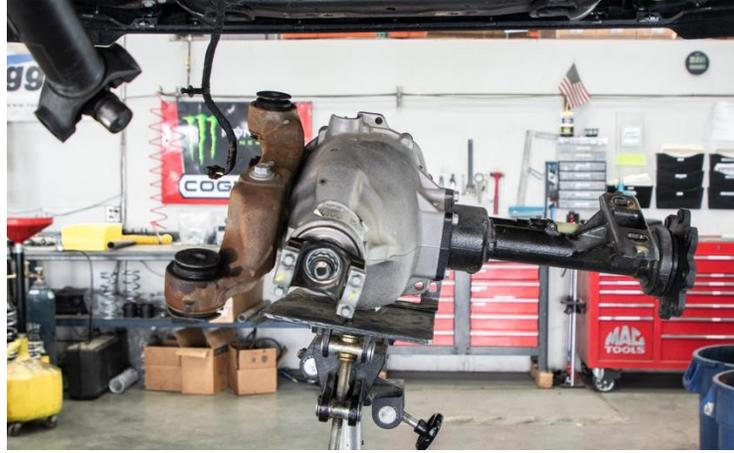
27. **Skip this step for 2WD vehicle.** After removing the differential from the vehicle, cut or grind a notch out of differential case. The notch will be made near the bolt hole closest to the yoke on the driver side of the differential. (See Figure 25)
