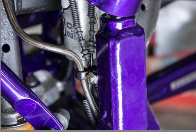
Figure 57: Driver Side Middle Spindle Tab & P-clamps
