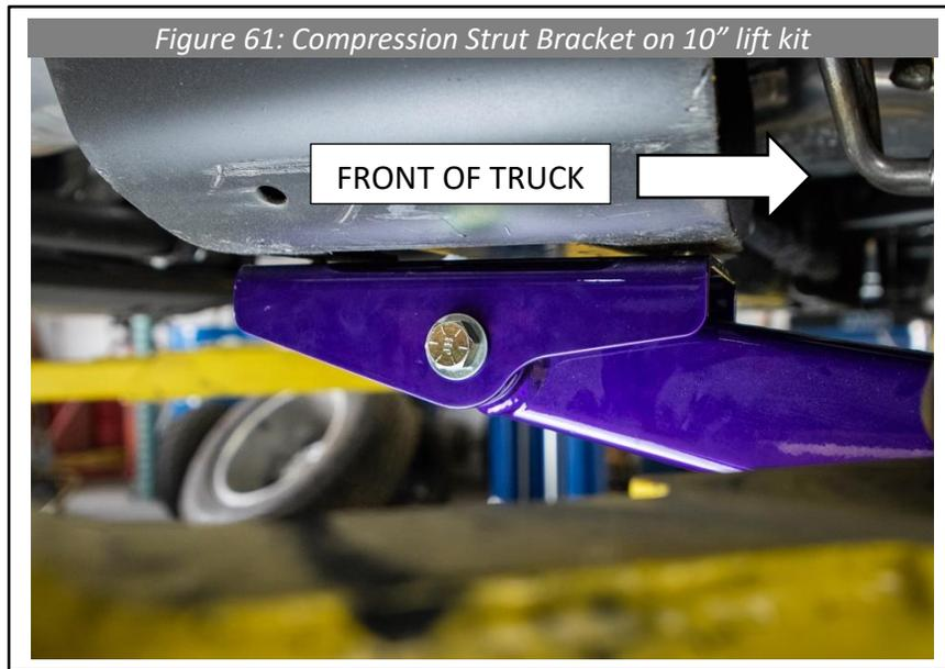
85. Swing the compression strut bracket up to the frame of the truck and be sure the mounting holes of the compression strut bracket line up appropriately to the factory frame cross member. If the mounting holes do not line up, test fit the other compression strut included in the kit. The pivot tube end near the rear crossmember is not welded perpendicular to the compression strut plates.
