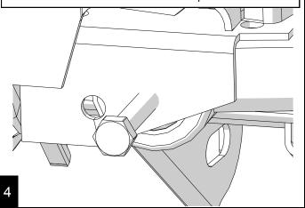
Insert the new 10mm x 75mm bolt. Torque to 40 ft-lbs.
