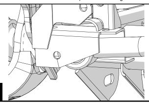
If you have room in the bracket so the hole does not overlap, go ahead and drill a hole with a 13/32" drill bit. If you drilled in the correct location the bar should line up with the new hole.
