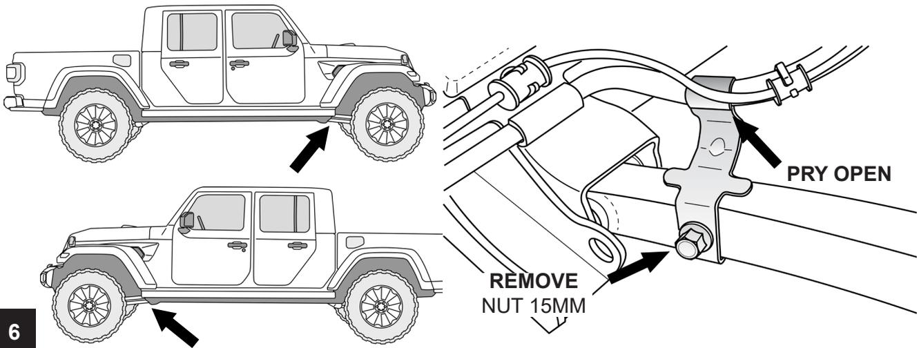
**DISCONNECT ACTUATORS AND VENT HOSE AT THE FRONT AXLE**
