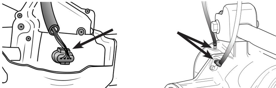
**RECONNECT PLASTIC RETAINERS FROM WIRING OR HOSES AS NEEDED.**
