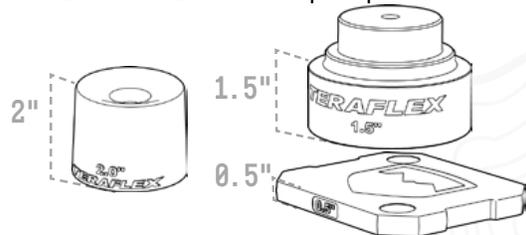
*Recommended Bump Stop configuration based on tested tires. Not all Tires Measure the Same. Cycling the suspension to check the shocks, springs and other suspension componets before driving is recommended.*
