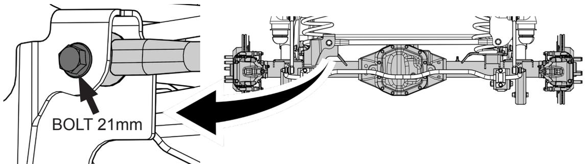
**LOOSEN BUT DO NOT REMOVE THE CONTROL ARM BOLTS**
