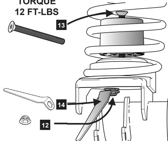
**WITH SPRINGS IN PLACE CHECK THE ISOLATOR AND SPACERS FOR CORRECT ALIGNMENT AND THAT THE SPRING IS FULLY SEATED INTO THE LOWER ISOLATOR**
