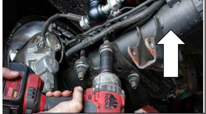
Support Axle Before Removing U-Bolts
