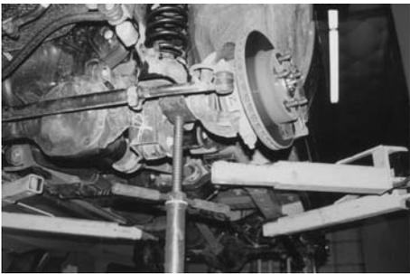
3. Before removing the springs, note how the spring sits in relation to the lower spring insulator. You will need to reposition the springs like this later. Remove the springs. Spring compressor are recommended to make this much easier. Spring compressors will make replacement easier too.
