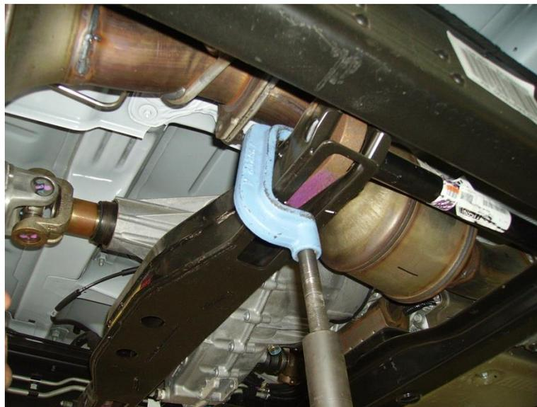
**Figure 2: load torsion bar to remove adjuster nut**
