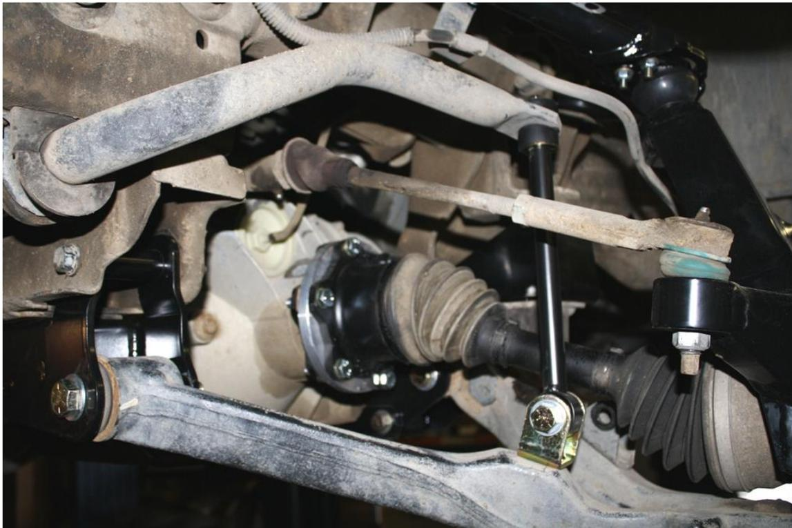
**Figure 25: Spindle, end link, axle, tie rod.**
