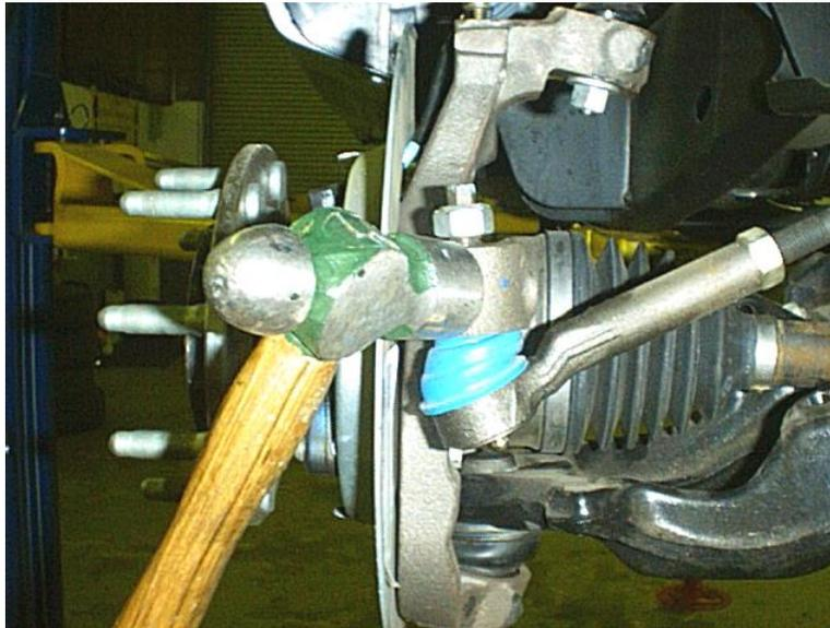
**Figure 7. Remove tie rods from spindles.**
