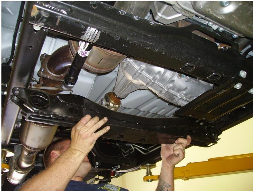
**Figure 4: Remove factory torsion bar crossmember**
