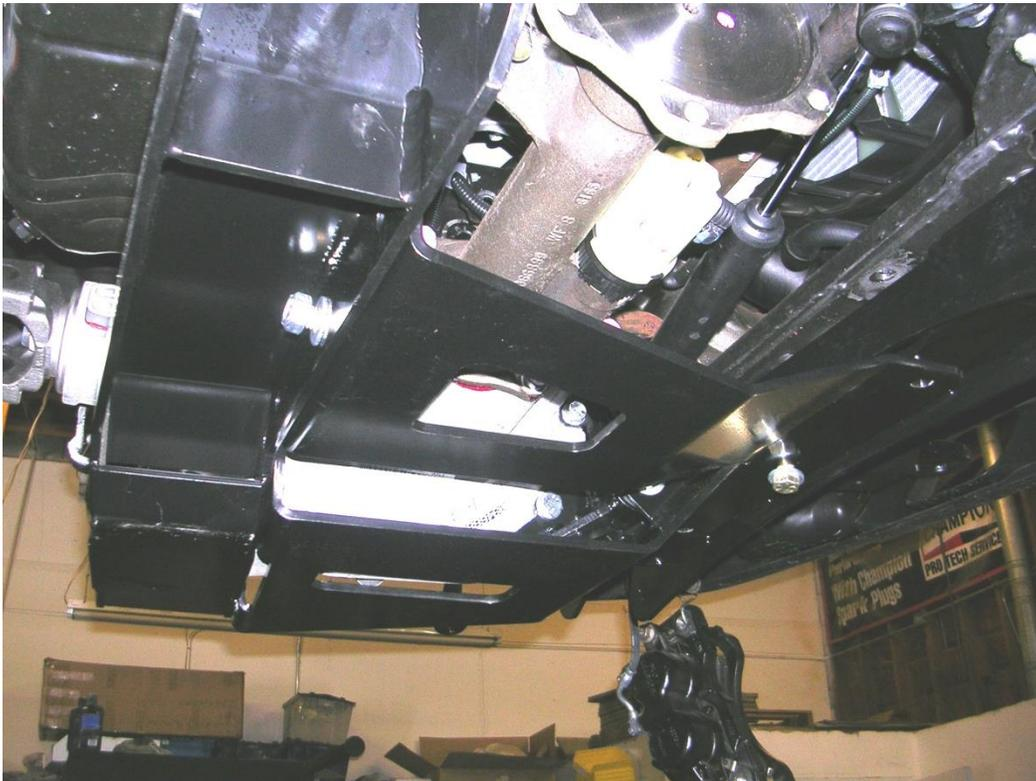
**Figure 22: Cognito Skid Plate during installation**
