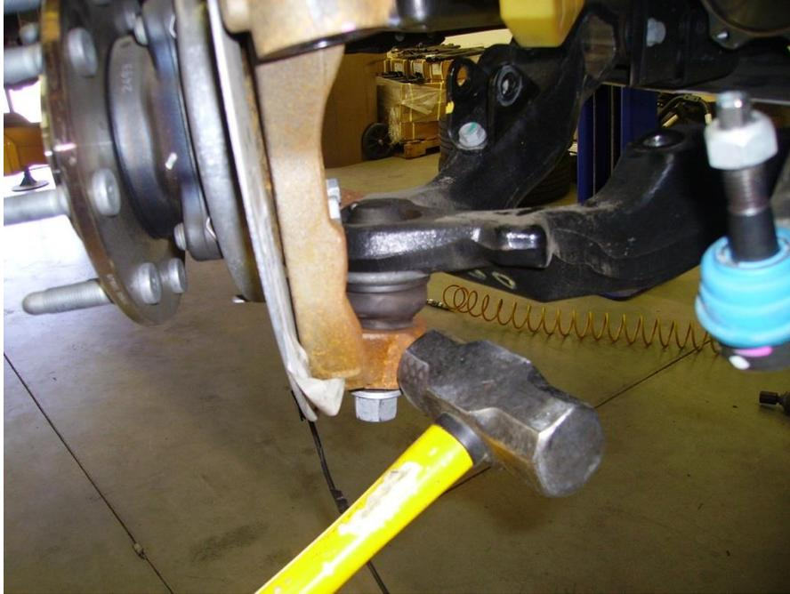
**Figure 9: removing lower control arm.**
