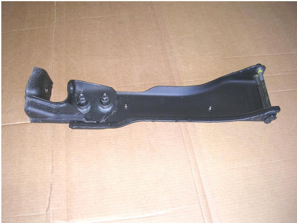
**Figure 15: Factory crossmember and frame section removed.**
