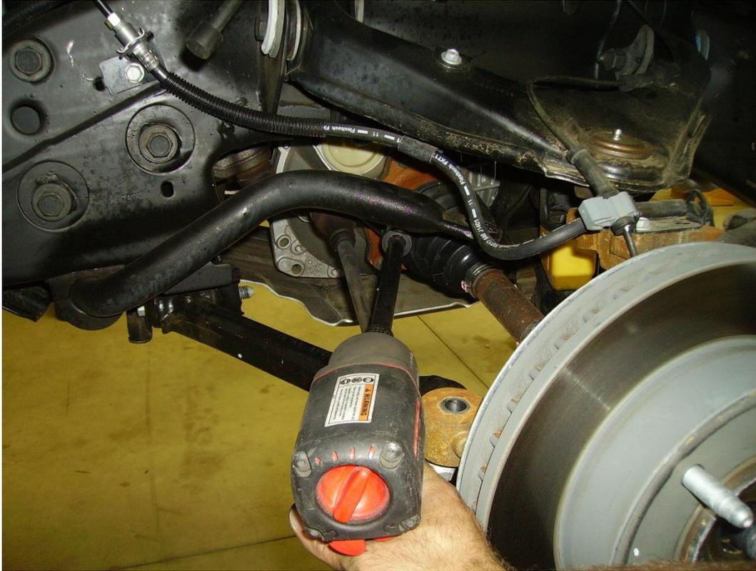
**Figure 8: Remove CV axles on 4wd vehicles**
