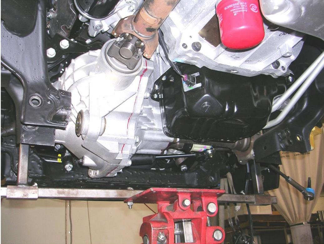
**Figure 14: Factory crossmember and frame section removed.**
