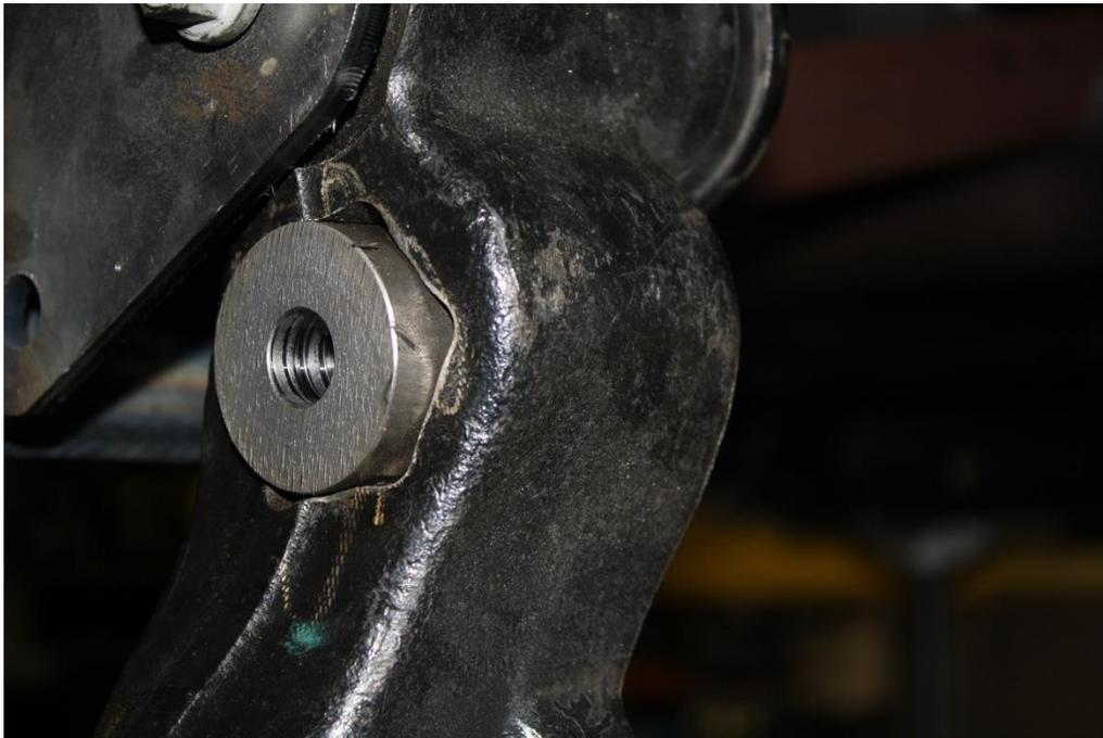
**Figure 26: 5388 mandrel inserted into lower control arm.**
