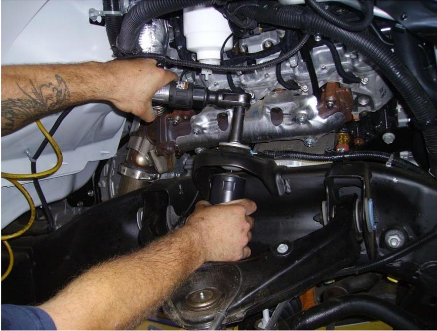
**Figure 5: remove shocks, front upper shown here.**
