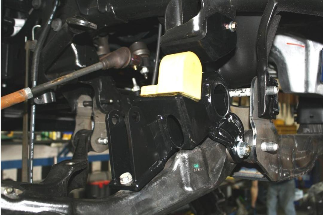
**Figure 27: 8213 bracket bolted to driver lower control arm.**
