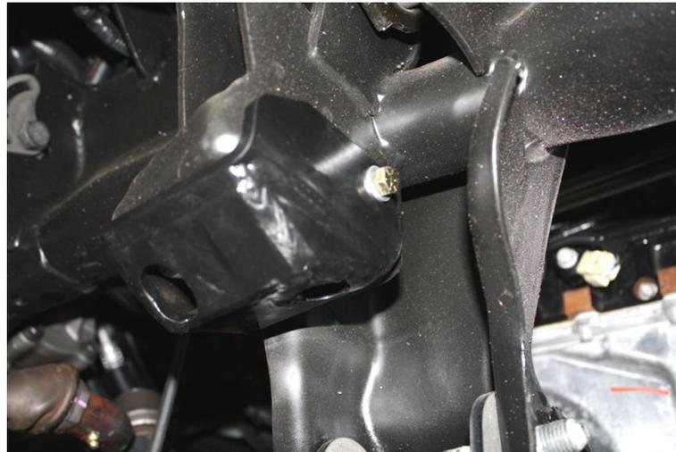
**Figure 20: bolt bump bracket to existing hole on side.**
