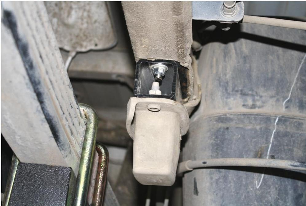
**Figure 28: Rear bump stop spacer**
