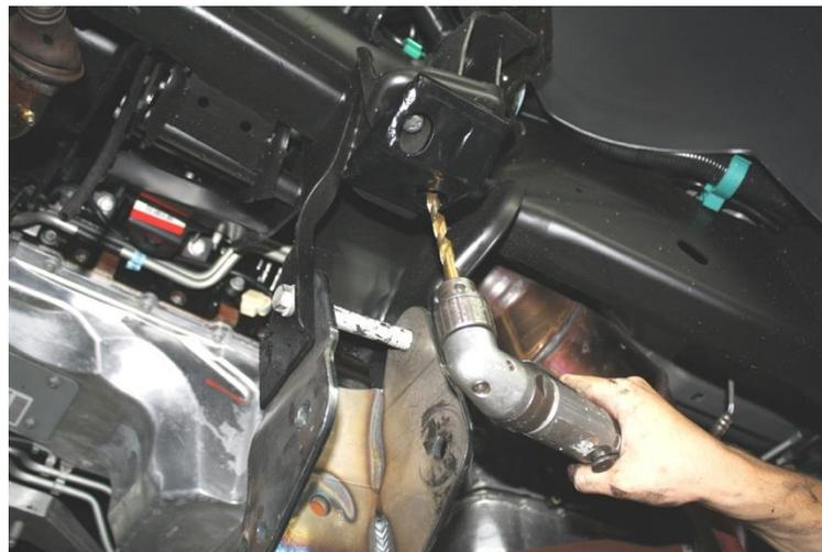
**Figure 12: drill mounting hole for bump stop brackets**
