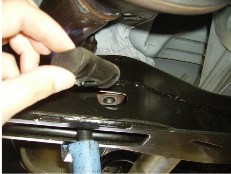
**Figure 3: adjuster nut removed**
