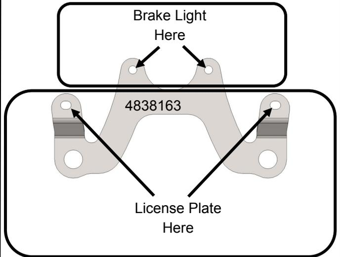
1. Install and tighten the supplied 1/2" bolts and lock washers through the brake light mount plate holes and into the long lug nuts. See the image below for the correct positioning of parts.
