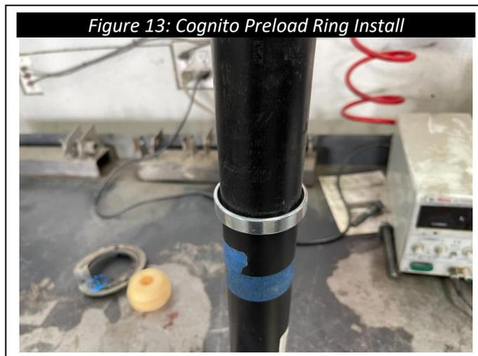
15. Install the factory spring seat over the Cognito preload ring, the shock rod seal cap by tapping it into place with a soft faced hammer, the nylon cover for the spring seat, and the foam bump stop cushion.
