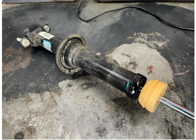
16. Reassemble the shock body and the strut assembly. Make sure to align the markings created in the prior step before tightening the center nut on the top of the strut assembly. Torque to **33 ft-lbs.**
