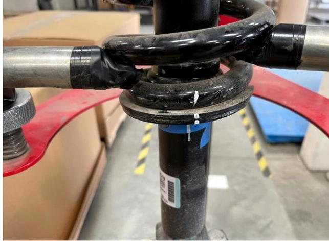
17. Locate **91037**, Cognito strut spacer, and **HP9270**. Install the spacer onto the strut and run the M10 nuts all the way down the studs but do not fully tighten. With a marker and straight edge, mark each stud level to the top plane of the spacer. Remove the nuts and spacer and double check the height of the mark made. The mark should be about  $1\frac{1}{16}$ " –  $\frac{3}{4}$ " above the plate where the studs come through the top hat.
