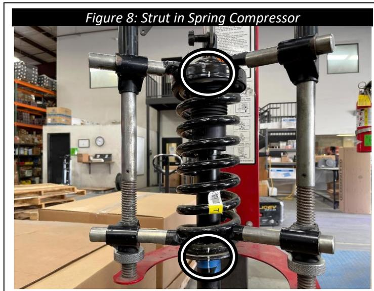
10. Using any form of spring compression tools, compress the strut assembly until the shock body assembly can spin freely. Remove the center nut at the top of the strut assembly using an impact gun and free the shock body assembly from the strut assembly.
