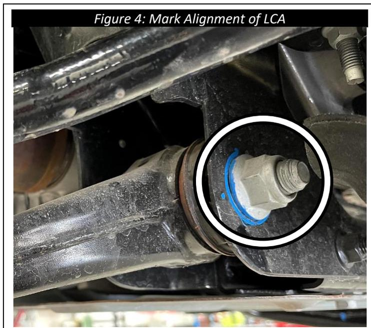
6. Remove the strut's two lower nuts underneath the LCA. Place the hardware safely aside, it will be reused later.
