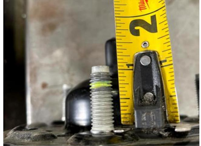
18. Using a cutting wheel, cut each of the studs off at the mark that was made in the step above.
