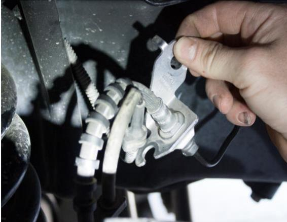
*Figure 3B: Driver ABS Line Removal*
