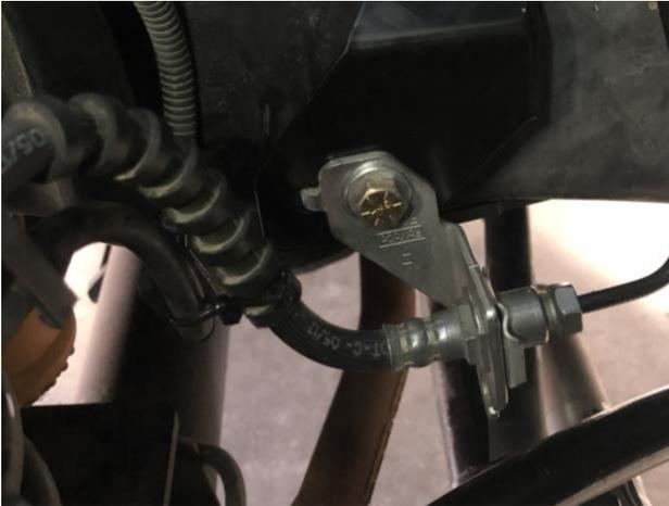
*Figure 7: Passenger Side ABS Line Routing*
