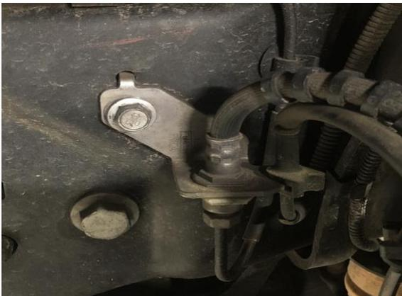
Figure 2B: OE Brake Line Bracket, Bolt Removed
