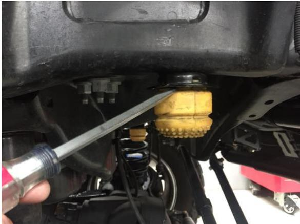
Figure 12B: FSD Bump Stop Spacer Hardware
