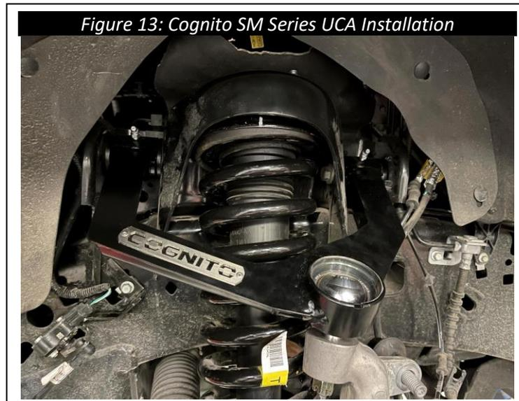
16. Mount the uniball pin to the spindle with the M12 castle nut. Use the flat washers supplied if the castle nut needs to be spaced down for the cotter pin to engage with its castellations. Torque the nut to **60 ft-lbs.** Install cotter pin and bend to lock into place.
