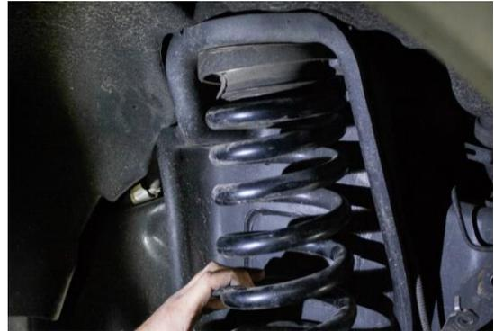
4. Locate the Cognito coil spring (COIL-SPRING-2003), and align the OE rubber isolator, removed in step 9, with the top spring pig-tail (Figure 14A). Install the spring with isolator onto the lower spring perch and rotate until the bottom spring pig-tail makes contact with OE spring perch tab (Figure 14B). Repeat for the opposing side of vehicle front spring.
