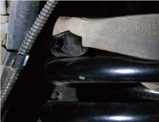
*Figure 14B: Bottom Spring Pig-tail Orientation*
