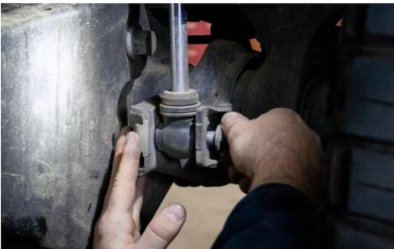
Figure 16B: Front Lower Shock Mount Installed
