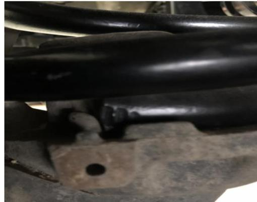
5. Once the springs are installed, locate the Cognito/FOX extended length shocks. Remove the top washer (Figure 15A) and bushing, then insert the top shock mounting stud through the frame, making sure the polyurethane pancake bushings are in place on both sides of frame. Install the top mounting washer with the concave side against bushing (Figure 15B). Repeat for the opposing side front shock, but do not tighten at this time.
