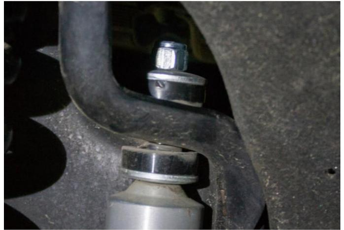
6. Before starting this step, it is recommended to get another person to assist you. Align both front shock bottom eyelets into lower shock mount shackle. Slowly lower the vehicle until the lower shock eyelets are aligned with the shackle mounting hole (Figure 16A). Re-install the OE bolt and locking nut plate, then torque to OE torque specifications (Figure 16B).
