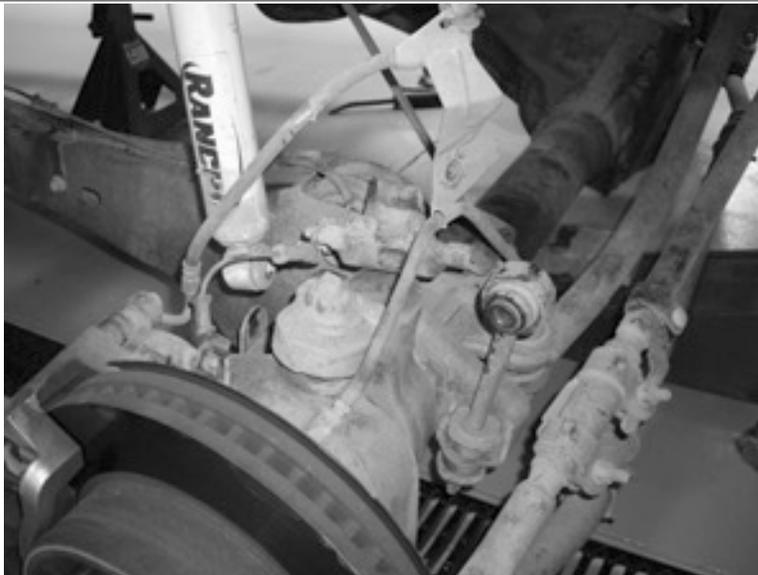
11. As shown in Figure 4, re-install the factory spring perch with the supplied coil spacer to space the perch above the housing from the stock location. Fasten the spacer and perch with the supplied bolt and lock washer and place a small amount of thread locker on the bolt, then torque to 100 ft. lbs. repeat on other side of vehicle.
