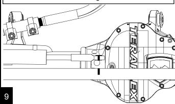
Apply blue thread locker to the threads of the 1/4" Socket Head Cap Screws. Install the clamp, centering the threaded bung on the mark. Note clamp orientation.
