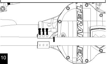
With a 15/16", install the remaining end of the ram onto the clamp using the 5/8" bolt and washer supplied by PSC. Apply blue thread locker and torque to 130 ft-lbs.
