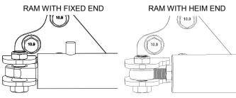
Reinstall the tie rod end nut and torque to 63 ft-lbs. If removed, reinstall the front tire.
