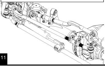
Have an assistant turn the steering wheel lock to lock. Verify that all components clear and that the ram's shaft does not bottom out or over extend before the steering stops make contact. Once clearance and position of the clamp have been verified, use a 3/16" Allen wrench to final tighten the 6 clamp bolts to 75 in-lbs. Tighten in a circular pattern.
