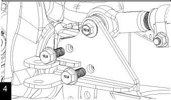
Using a 21mm, loosen the passenger side tie rod end nut, but do not remove. Leave the nut threaded on a few turns to protect the threads and prevent the tie rod from falling when it releases.
