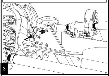
Install the two M14 bolts with the lock washer positioned between the nut and the bracket. Apply red thread locker. Torque all hardware to 125 ft-lbs using a 21mm and 22mm..
