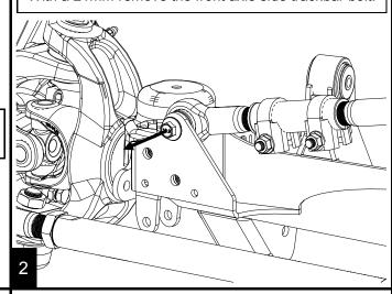
Begin mounting the hydro assist ram bracket by installing the supplied track bar hardware. Finger tighten.
