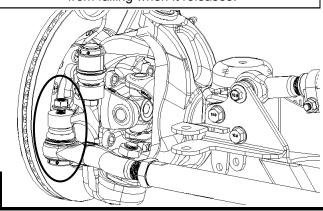
With a hammer, strike the knuckle casting just above the tie rod until the tie rod breaks free. Do not hit the tie rod or the tie rod end directly. Hint, remove the front tire for better access.
