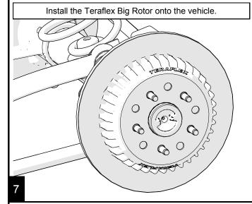
For slotted rotor applications, install the rotors in the orientation shown.
