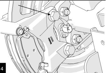
Remove the caliper slides from the factory bracket by pulling them out of their factory bores. Apply a dab of caliper slide grease into the slide bore of the new caliper bracket.
