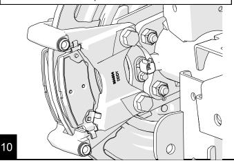
Install the factory caliper using the original bolts and a thread locking compound. Torque to 30 ft-lbs.
