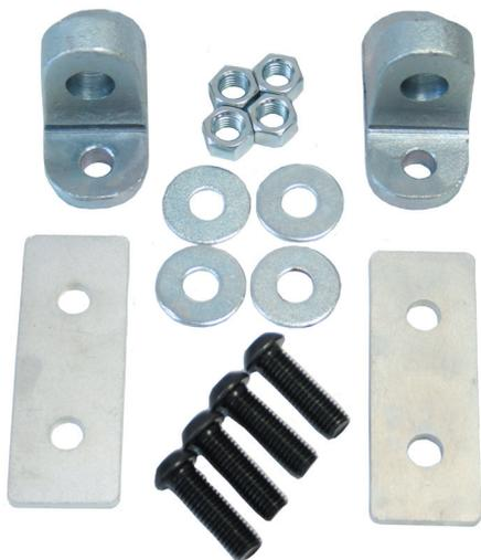
Place D-ring mounts on the front of the TJ front bumper using the bolts provided. Bolt them to the bumper using the pre-drilled holes. Place backing plates on the inside of the bumper sliding them onto the backside of the bolts holding the D-ring followed by the washer and nuts.
