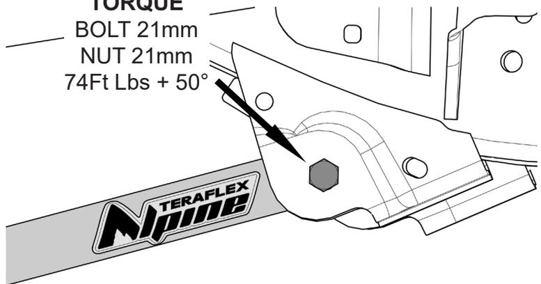
LOOSEN THE CLAMP AND EXTEND THE CONTROL ARM TO THE RECOMMENDED LENGTH. INSTALL THE CONTROL ARM INTO THE AXLE MOUNT.
