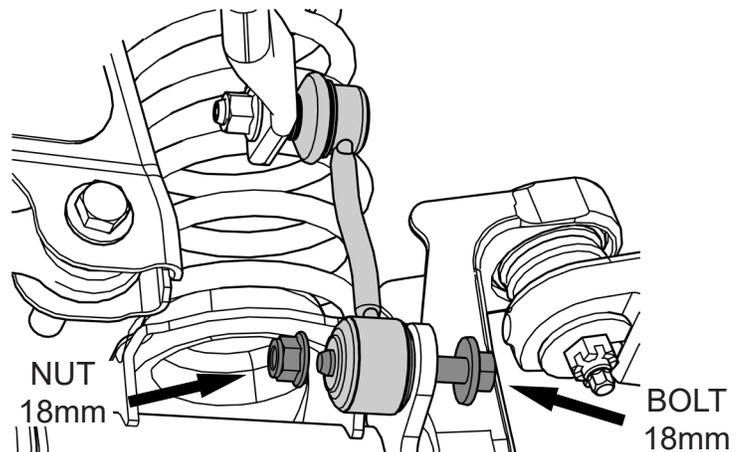
**REMOVE THE FRONT LOWER SHOCK BOLTS AND REPLACE WITH THE LOWER SWAY BAR LINK BOLTS**
