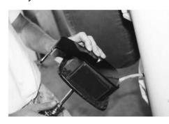
Position the antenna mounting bracket between the vehicle and the tail light housing. The mounting portion of the bracket will be positioned towards the outside edge of the tail light housing when properly installed.
