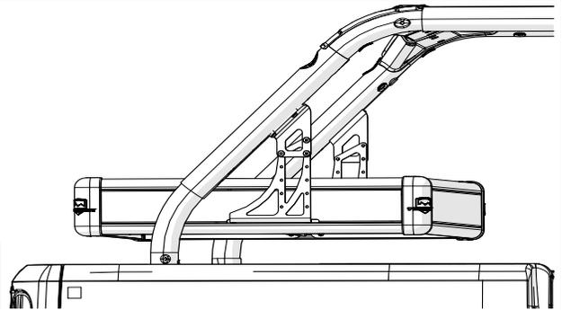
The rack is adjustable both vertically as well as front to back. Slide the rack forward until there is a 1/4" gap between the rack and back seat. Torque the bolts to 5 FT-LBS (7 Nm).
