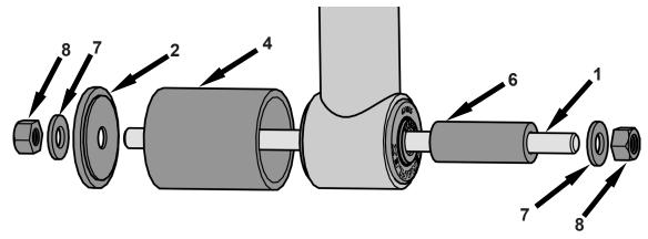
USING A 19mm SOCKET AND WRENCH TIGHTEN THE ASSEMBLY UNTIL THE BUSHING IS REMOVED FROM THE CONTROL ARM
