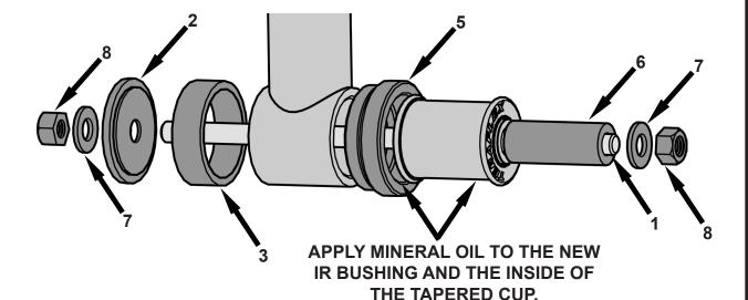
USING A 19mm SOCKET AND WRENCH TIGHTEN THE ASSEMBLY UNTIL THE BUSHING IS INSTALLED INTO THE CONTROL ARM
