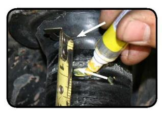
8. Cut the jounce tube with a cut off wheel, this cut is made to locate the hole saw. You may need to pry the jounce tube towards the frame to completely cut through the tube.
