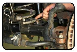
Once bolts are removed, lower jack so the front springs can be removed. If springs are still tight and will not come out you can remove more suspension components like sway bar links and track bar.
