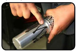
17. Install the Speedbump into the mount. Place the collar on top and use a 3/16" allen to torque the pinch bolt. Wipe the excess silicon away with a damp cloth.
