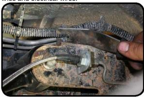
24. Cut off the old coil perch using a torch or cut off wheel.
