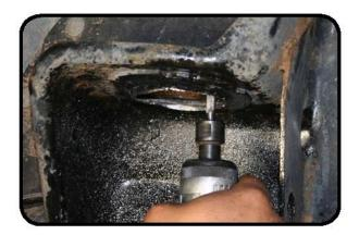
11. After you have cut though both layers grind the jounce tube flat to ensure a good fit and weld with the new Speedbump bracket.
