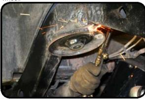
25. Grind the frame flush so that the new TeraFlex Speedbump coil perch mounts correctly.
