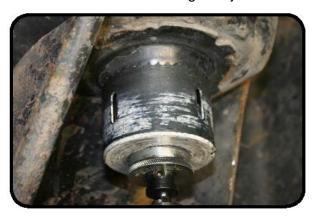
10. You may need to use a die grinder to open up the hole to get the hole saw to cut through the second layer.
