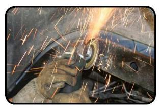
26. Jack up on the axle to locate where the new coil perch needs to mount. Place the mount on the frame and align it so that the Speedbump will contact the center of the spring perch.
