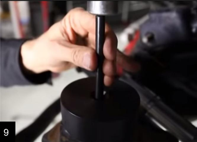
Drill a 3/8" hole; We recommend first drilling a pilot hole. Set the strike pad in place for measurements.
