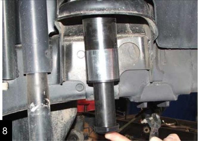
Remove the speedbump and center the strike pad on the spring perch. Use a center punch through the hole to mark the center.
