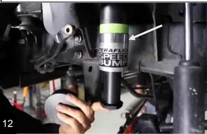
With the necessary shims in place, apply a coat of silicone sealant (not adhesive) over the cylinder of the Speedbump where it will be in contact with the factory tube.
