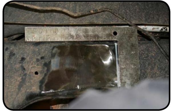
5. Measure 2 1/2" forward from the rear scribe line. Mark and use a square to mark the area that will be removed.
