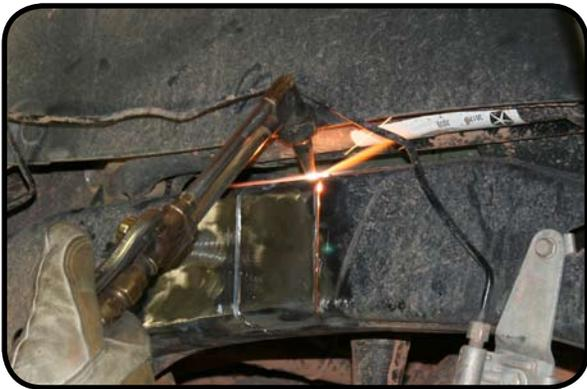
9. Remove the piece of the frame and grind to fit the new speedbump mount.
