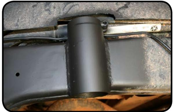
12. Reroute the brake line behind the speedbump mount. You will need to straighten the brake line to do so.
