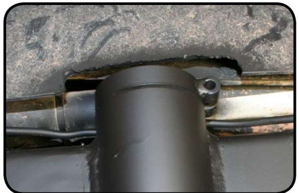
14. Install the TeraFlex speedbump into the new mount. Use silicon on the speedbump and slide it up into the mount. Use the supplied bolt to tighten the pinch clamp.
