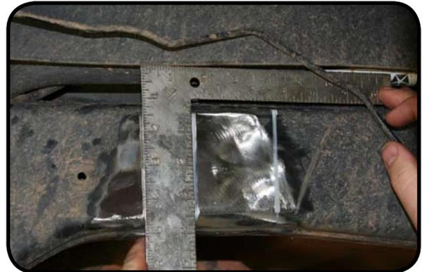
6. The depth of the cut needs to be 1 1/8" on the top and bottom of the frame. This should put the new speedbump mount flush with the coil bucket weld on the top of the frame. (Use the arrows below for reference. View from the top of the frame.)
