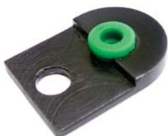
10. Re-attach the transfer case linkage bracket to the bottom of the tub. Attach the linkage with bracket to the transfer case.
