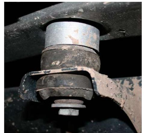
5. Replace the stock bolt taken out with the new included bolt, but do not tighten the bolts yet.
