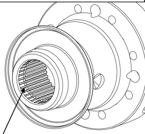
Apply blue thread locking compound to the shaft threads and install the yoke. Reinstall the O-ring and torque the factory yoke nut. Front- 90-130 ft-lbs (122-176 Nm) Rear- 190-230 ft-lbs (258-312 Nm).
