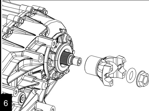
Apply a bead of silicone to the back side of the splines on the new yoke and install onto the output shaft.
