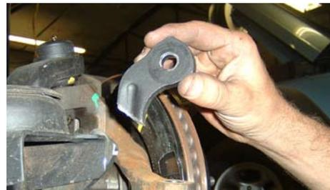
2. Grind the area smooth to avoid cutting yourself on the sharp edge, and paint to prevent rusting.
